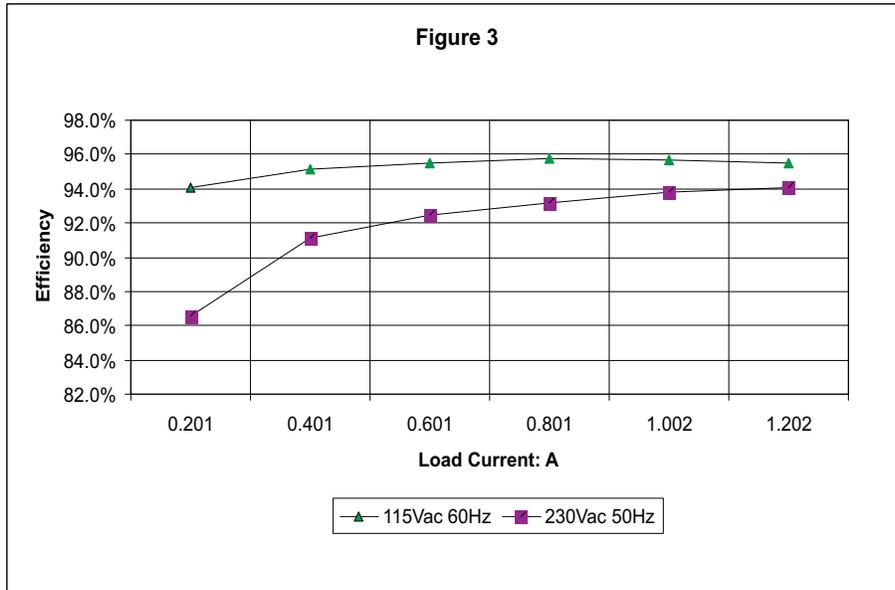
Figure 3. Efficiency with 115 V<sub>AC</sub> and 230 V<sub>AC</sub> (Test Points: TP1, TP2, TP12 and TP13)
