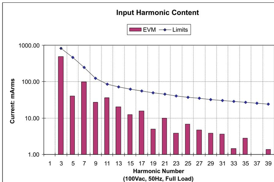
Figure 8. Harmonic Content with 100 V<sub>AC</sub> Input ( $V_{IN} = 100 V_{AC}$  at 50 Hz,  $I_o = 1.2 A$  Test Points: TP1, TP2, TP12 and TP13)
