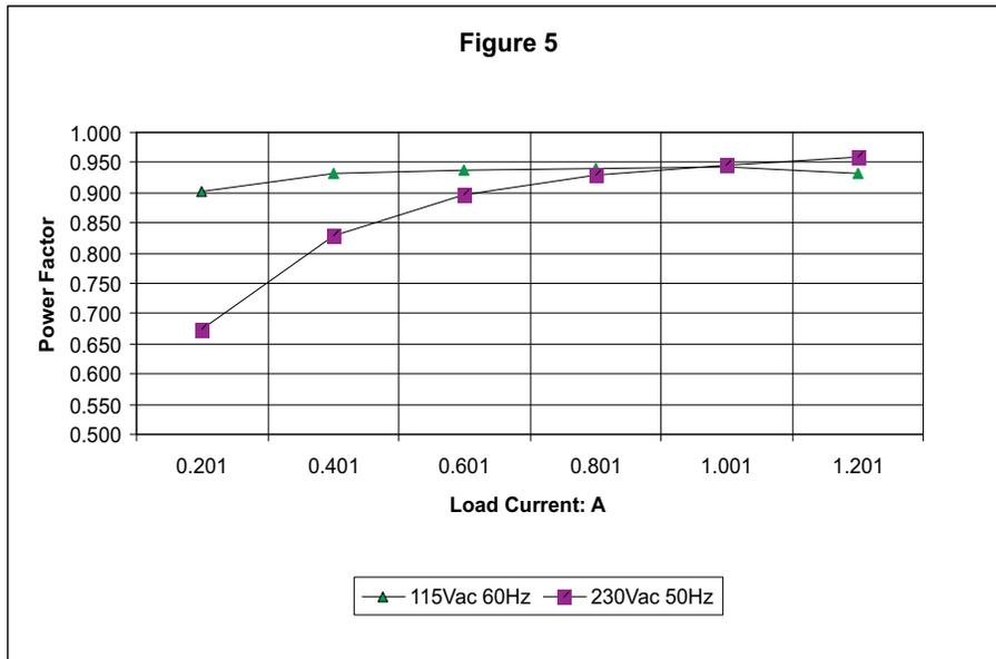
Figure 5. PF with 115 V<sub>AC</sub> and 230 V<sub>AC</sub> (Test Points: TP1, TP2, TP12 and TP13)
