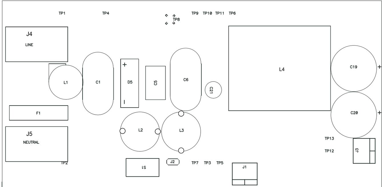
Figure 13. UCC29910AEVM-730 Top Layer Assembly Drawing (top view)
