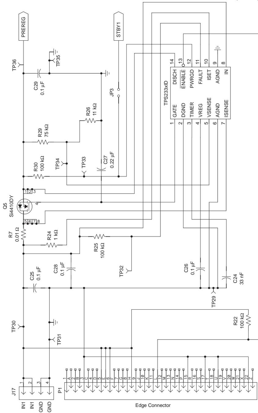
NOTE: A 14-V Zener diode in parallel with C25 is recommended for noisy applications to limit the input voltage within the operation range of TPS2331
