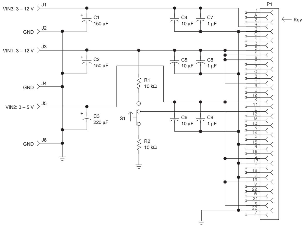
Figure 3–2. Schematic of the InfiniBand Bulk Power Evaluation Module (EVM) (Part 1)
