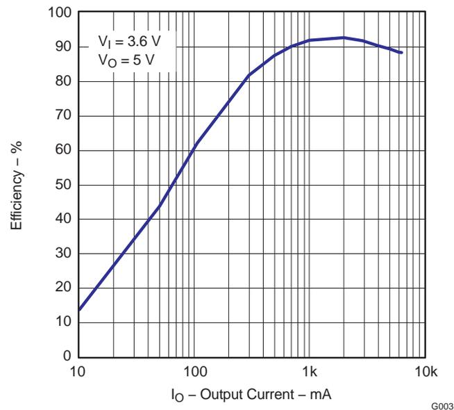
Figure 5. Voltage-Mode Efficiency
