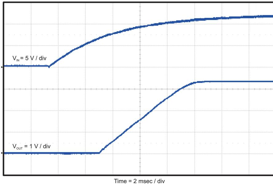
Figure 9. TPS54622EVM-012 Start-Up Relative to  $V_{IN}$
