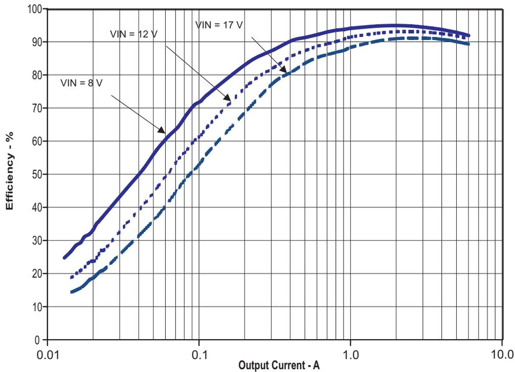
Figure 2. TPS54622EVM-012 Low Current Efficiency
