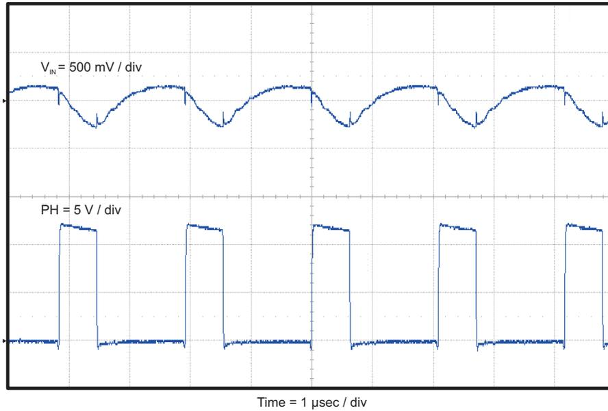
**Figure 8. TPS54622EVM-012 Input Ripple**
