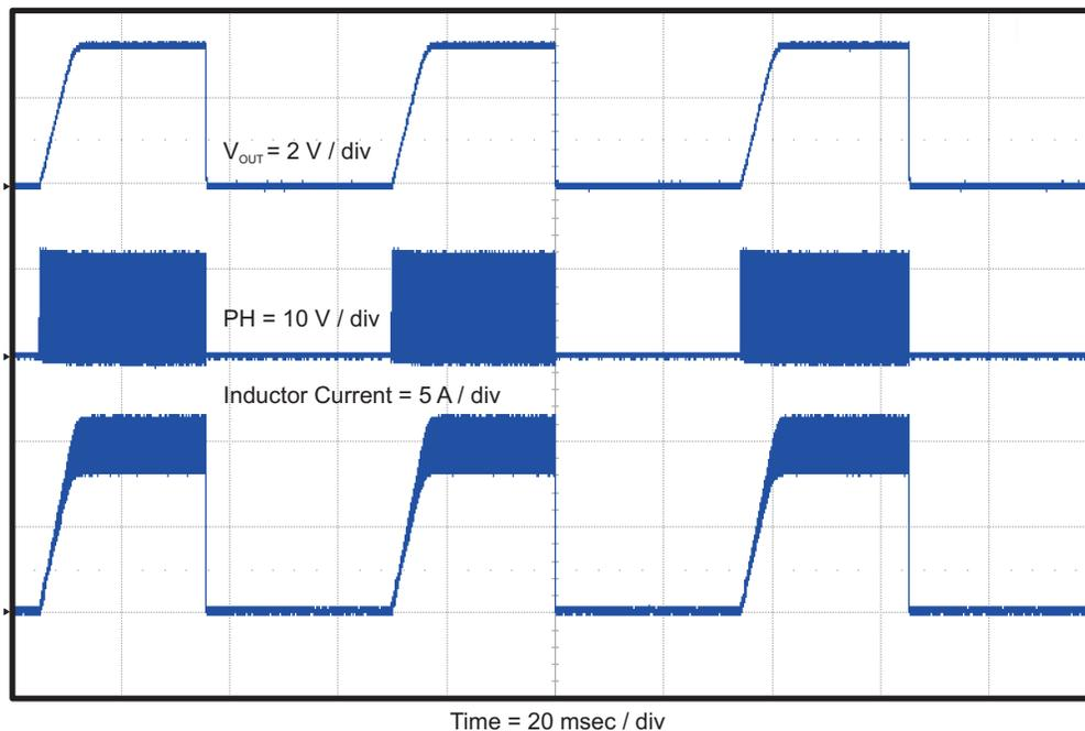
Figure 12. TPS54622EVM-012 Hiccup Mode Current Limit
