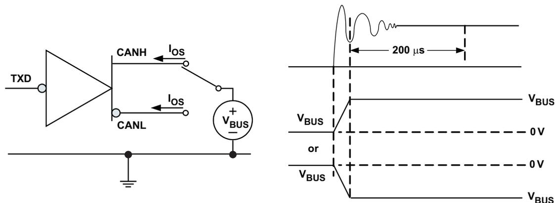
Figure 15. Driver Short Circuit Current Test and Measurement
