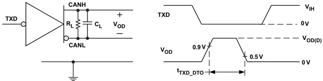
Figure 14. TXD Dominant Timeout Test Circuit and Measurement
