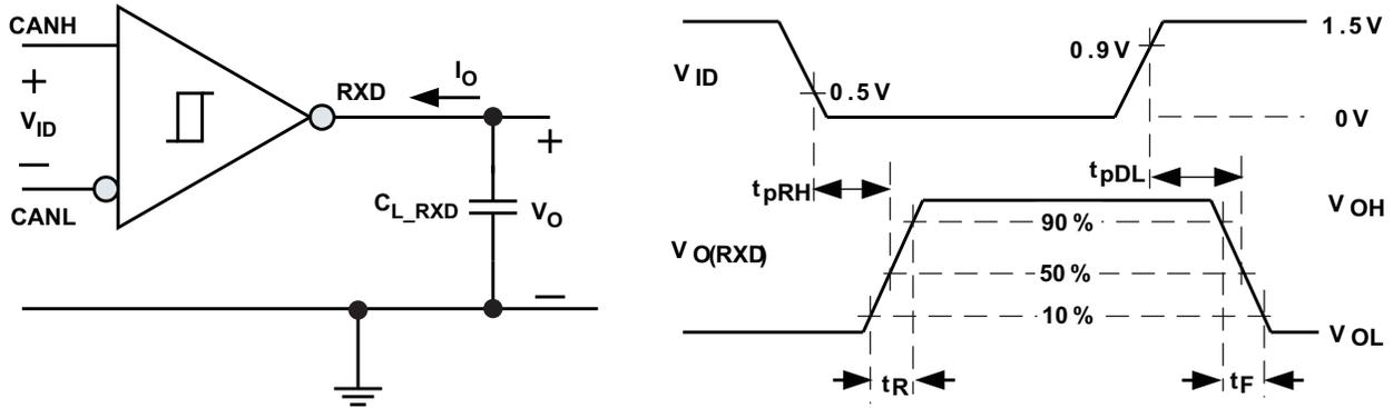
Figure 11. Receiver Test Circuit and Measurement
