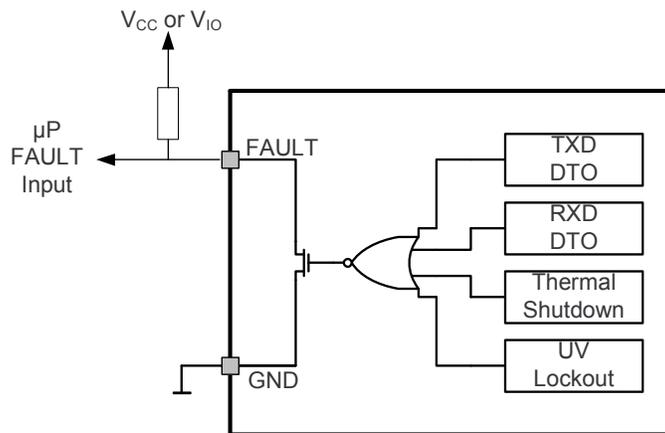
**Figure 5. FAULT Pin Function Diagram and Application**
