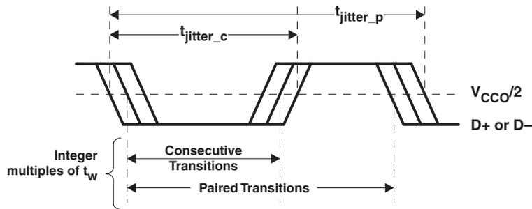
Figure 3. Output Jitter
