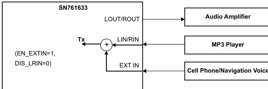
**Figure 29. Mixing Mode of Tx Signal**
