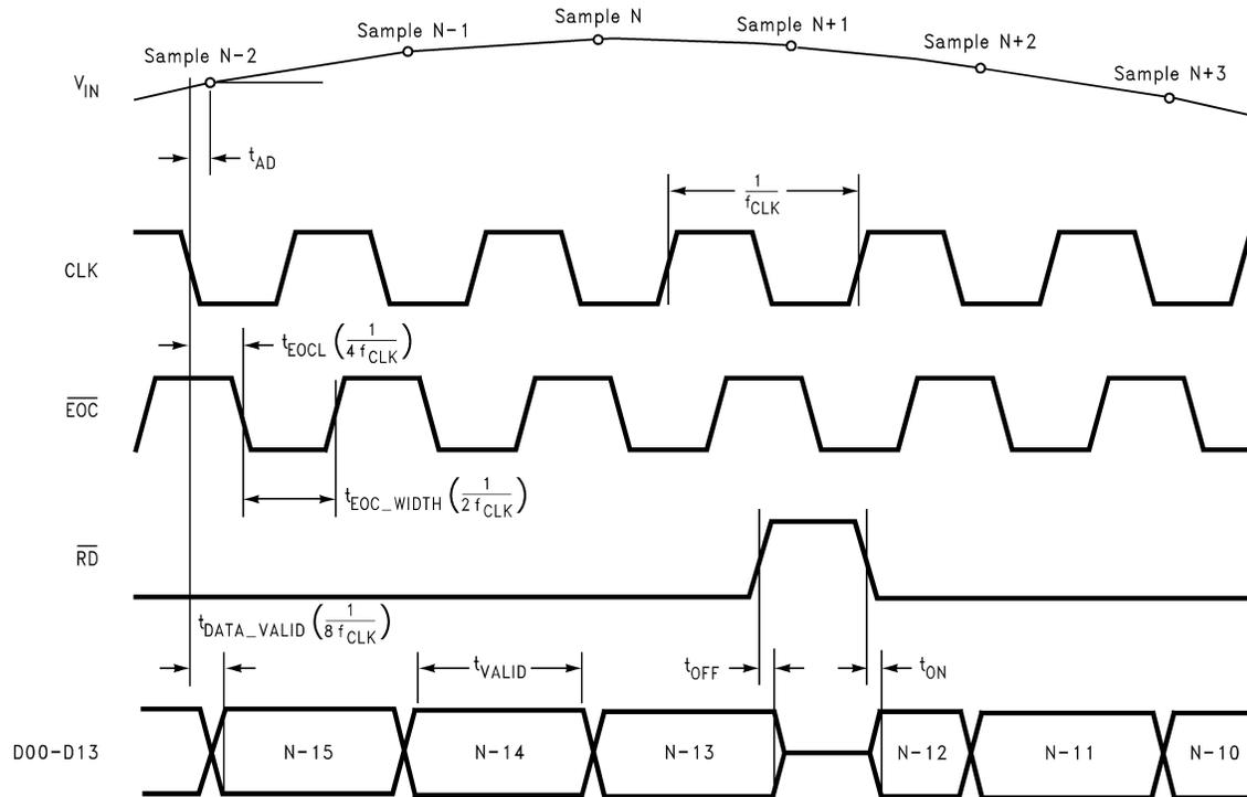
Figure 14. TIMING DIAGRAM 1. Output Timing
