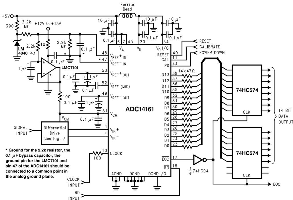
Figure 19. Simple application circuit with single-ended to differential buffer.
