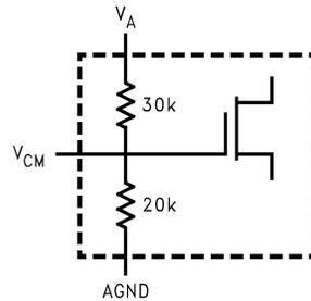
**Figure 18.  $V_{CM}$  input to the ADC14161  $V_{CM}$  is set to 40% of  $V_A$  with on-chip resistors. Performance is improved when  $V_{CM}$  is driven with a stable, low impedance source**
