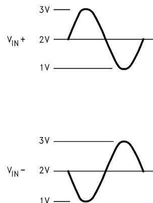
Figure 17. Expected Input Signal Range.
