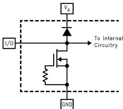
Figure 1. ESD Protection Scheme for Digital Input pins
