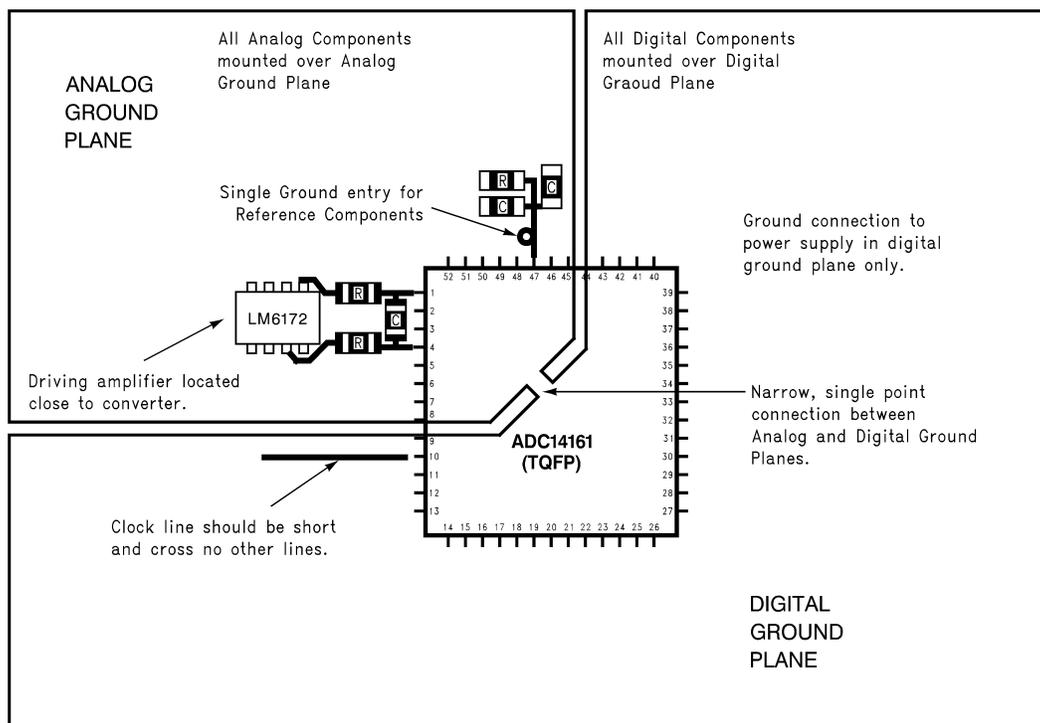
Figure 22. Example of a suitable layout
