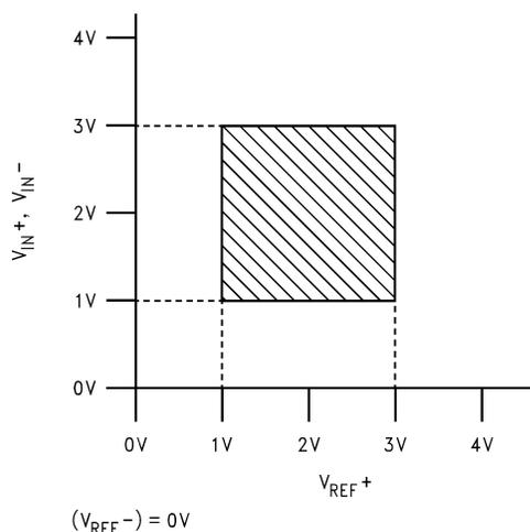
Figure 16. Typical Input to Reference Relationship.
