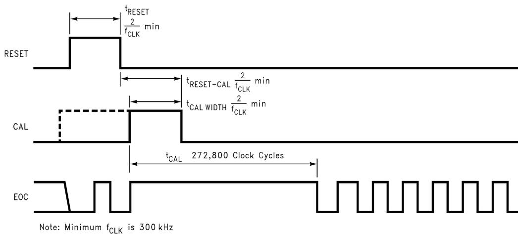
Figure 15. TIMING DIAGRAM 2. Reset and Calibration
