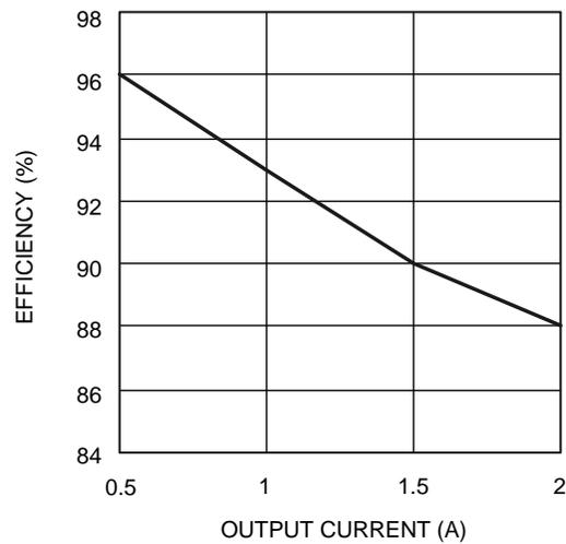
**Figure 2. Efficiency vs Output Current ( $V_{IN} = 5\text{ V}$ )**
