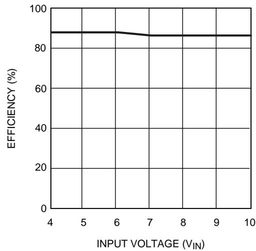
**Figure 3. Efficiency vs Input Voltage ( $I_{out} = 2\text{ A}$ )**
