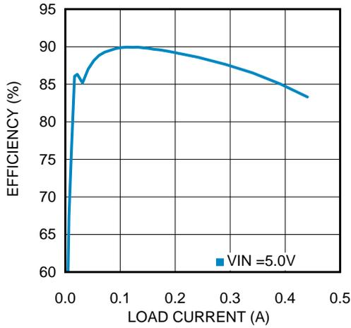
Efficiency vs. Load Current LMR62014, VOUT = 12V
