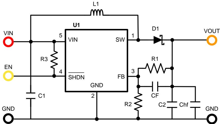
**Figure 2. LMR62014 Demo Board Schematic**
