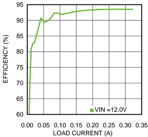
Efficiency vs. Load Current LMR64010, VOUT = 24V
