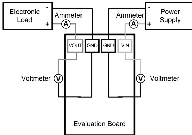
**Figure 4. Efficiency Measurements**
