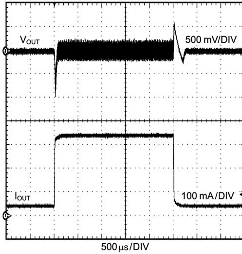
Load Transient Waveforms LMR64010
