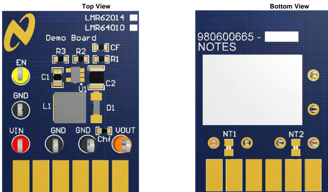
**Figure 1. LMR62014/LMR64010 Demo Board**
