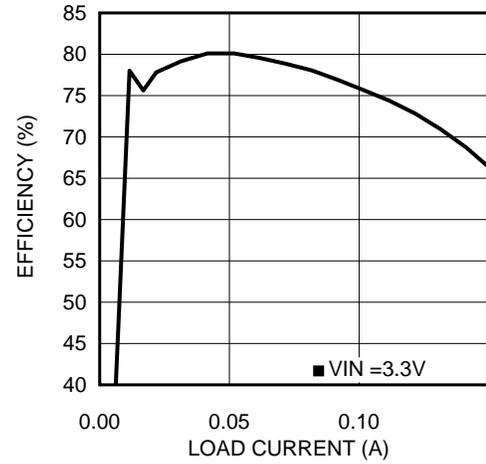
Efficiency vs. Load Current LMR64010, VOUT = 24V
