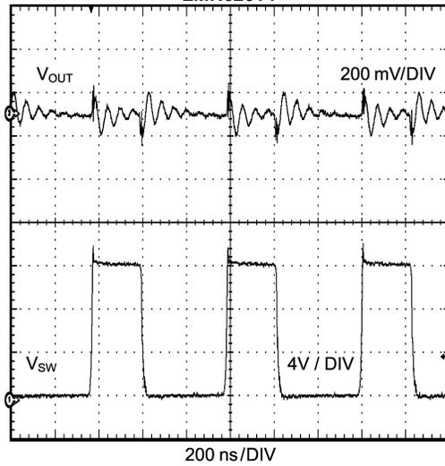
Switching Node and Output Voltage Waveforms
