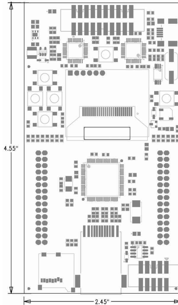
Figure B-3. LM3S2110 CAN Device Board Dimensions
