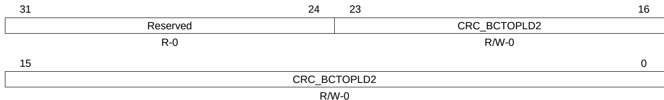
Figure 14-34. CRC Channel 2 Block Complete Timeout Preload Register B (CRC_BCTOPLD2) [offset = 90h]
