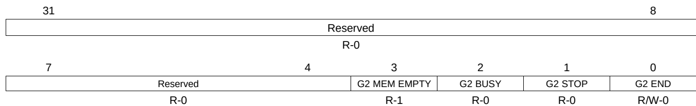
Figure 19-46. ADC Group2 Status Register (ADG2SR) [offset = 74h]
