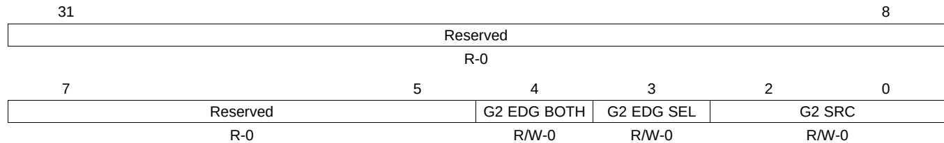
Figure 19-26. ADC Group2 Trigger Source Select Register (ADG2SRC) [offset = 24h]
