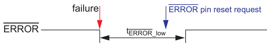
Figure 11-5. \overline{\text{ERROR}} Pin Timing - Example 2
