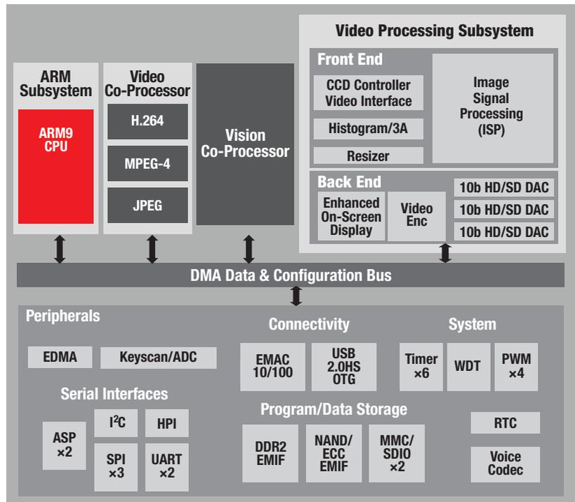
Figure 3: DMVA2 block diagram.
