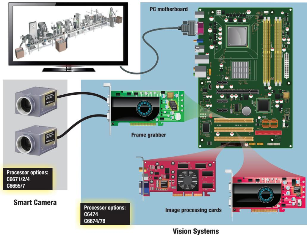
Figure 5: Typical industrial imaging system.
