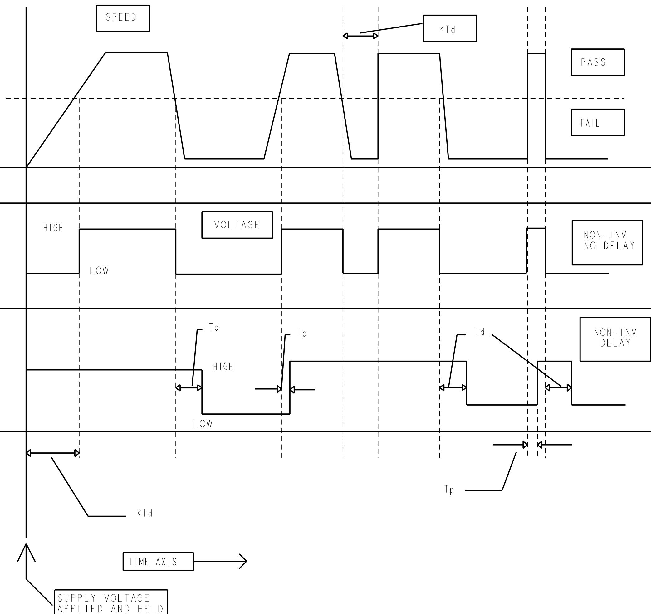
TD is the time delay after the pulses/min. go below the trip point. TD is set by the external RC.
