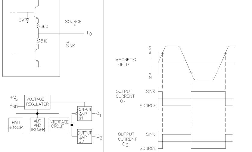
THE MAGNETIC FLUX USED TO OPERATE THE SWITCH MUST BE IN THE DIRECTION AND LOCATION SHOWN (THIS ASSUMES THE CONVENTION THAT THE DIRECTION OF THE EXTERNAL FLUX OF A MAGNET IS FROM THE NORTH TO THE SOUTH POLE OF THE MAGNET)
