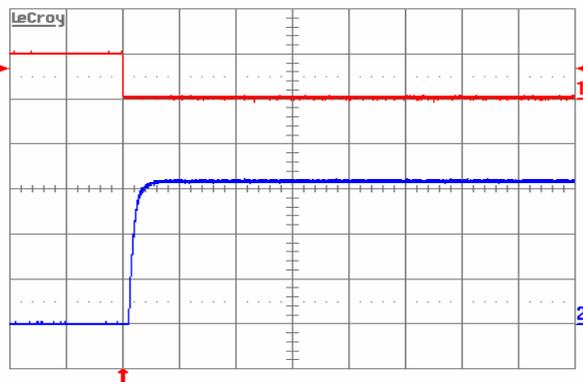
Figure 6. Turn-on transient at full rated load current (resistive) with no output capacitor at  $V_{in} = 48\text{ V}$ , triggered via ON/OFF pin. Top trace: ON/OFF signal (5 V/div.). Bottom trace: Output voltage (1.0 V/div.). Time scale: 5 ms/div.
