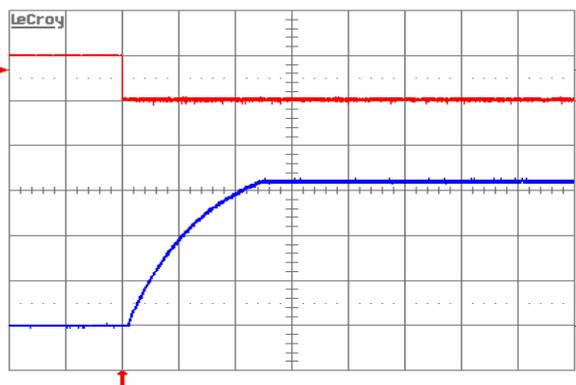
Figure 7. Turn-on transient at full rated load current (resistive) plus 20,000  $\mu\text{F}$  at  $V_{in} = 48\text{ V}$ , triggered via ON/OFF pin. Top trace: ON/OFF signal (5 V/div.). Bottom trace: Output voltage (1 V/div.). Time scale: 5 ms/div.
