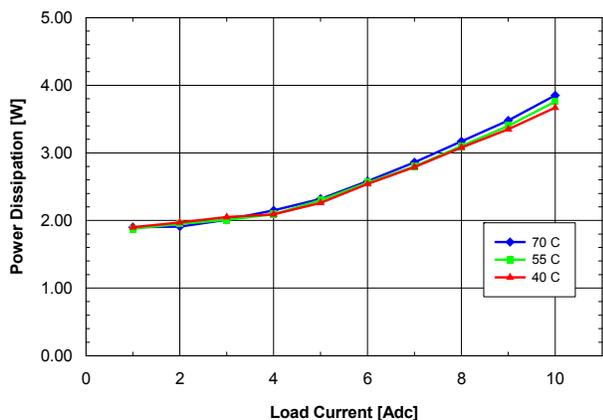
Figure 5. Power dissipation vs. load current and ambient temperature for SSQE48T10033 converter mounted vertically with  $V_{in} = 48\text{ V}$  and air flowing from pin 1 to pin 3 at a rate of 200 LFM (1.0 m/s).
