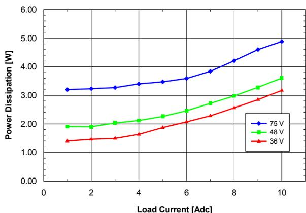
Figure 4. Power dissipation vs. load current and input voltage for SSQE48T10033 converter mounted vertically with air flowing from pin 1 to pin 3 at a rate of 300 LFM (1.5 m/s) and  $T_a = 25\text{ }^\circ\text{C}$ .
