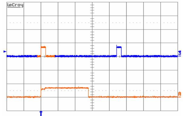
Figure 15. Load current (top trace, 20 A/div., 50 ms/div.) into a  $10 \text{ m}\Omega$  short circuit during restart, at  $V_{in} = 48 \text{ V}$ . Bottom trace (20 A/div., 5 ms/div.) is an expansion of the on-time portion of the top trace
