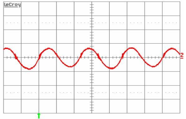
Figure 13. Input reflected ripple-current,  $i_c$  (100 mA/div.), measured at input terminals at full rated load current and  $V_{in} = 48 \text{ V}$ . Refer to Figure 11 for test setup. Time scale:  $1 \mu\text{s}/\text{div}$ .
