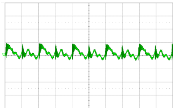
Figure 13. Output voltage ripple (20 mV/div.) at full rated load current into a resistive load with C_o = 10\mu\text{F} tantalum + 1\mu\text{F} ceramic and V_{in} = 48\text{V} . Time scale: 2 μs/div.
