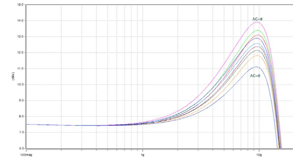
Figure 5 shows the Stratix V DC gain curves for GT channels.
