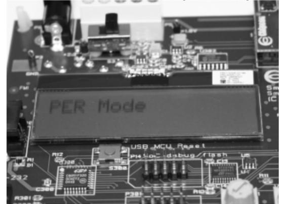
The Sender will show "PER Mode". The Sender will send a request to the Receiver to send it 1000 packets. It will then calculate the PER rate.
