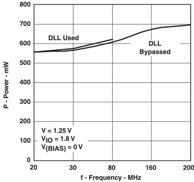
**Figure 7-4. Power vs Frequency**
