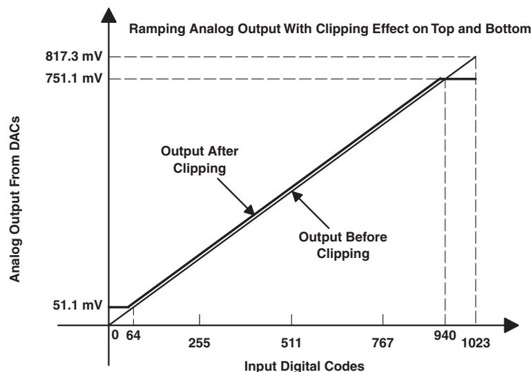
Figure 4-5. Effect of Clipping on Analog Output
