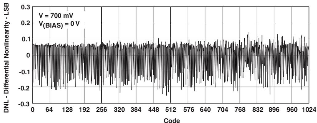
Figure 7-6. Differential Nonlinearity vs Code
