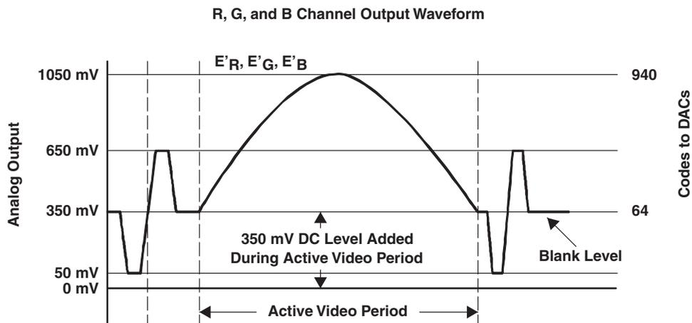
Figure 4-43. R-, G-, and B-Channel Output Waveform
