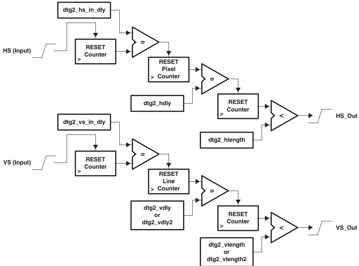
**Figure 4-15. THS8200 DTG VS/HS Output Generation**
