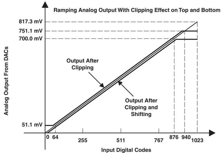
**Figure 4-6. Effect of Shifting on Clipped Analog Output**
