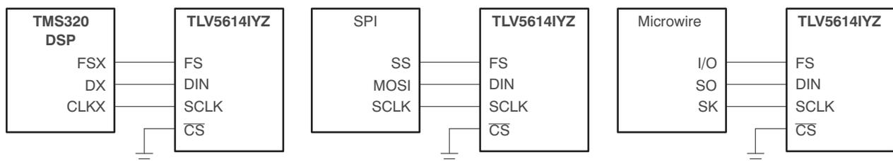
Figure 16. Three-Wire Interface
