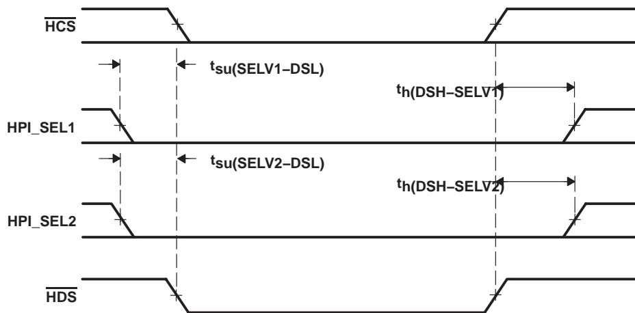
Figure 5-19. HPI_SEL1 and HPI_SEL2 Timing
