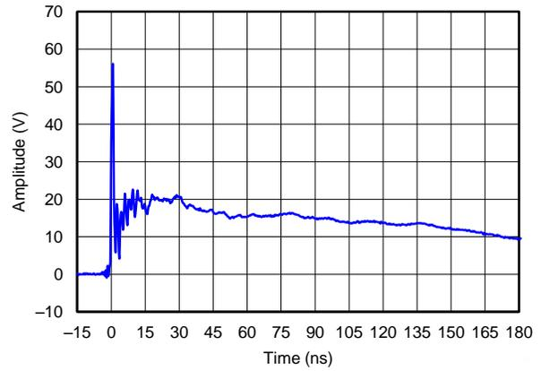
**Figure 7. IEC 61000-4-2 Clamping Voltage, +8kV Contact**
