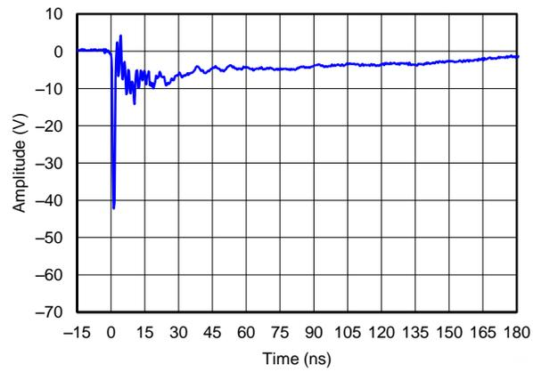
**Figure 8. IEC 61000-4-2 Clamping Voltage, -8kV Contact**
