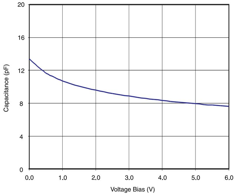
**Figure 1. IO Capacitance vs IO Voltage**
