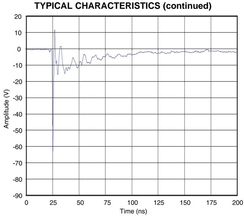
Figure 5. IEC Clamping Waveforms -8 kV Contact
