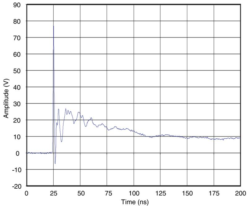
**Figure 4. IEC Clamping Waveforms 8 kV Contact**
