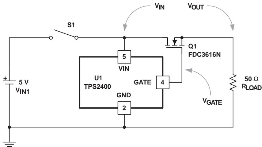
Figure 7. Output Turn-On Response Test Circuit
