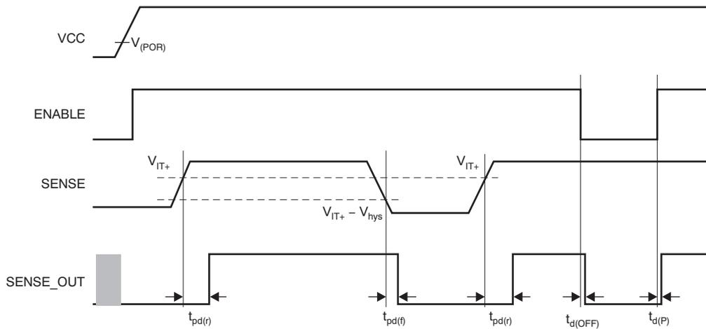
Figure 2. TPS3895P/TPS3897P Timing
