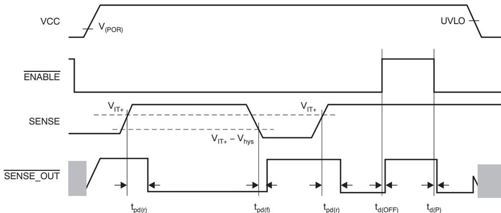
Figure 4. TPS3896P/TPS3898P Timing
