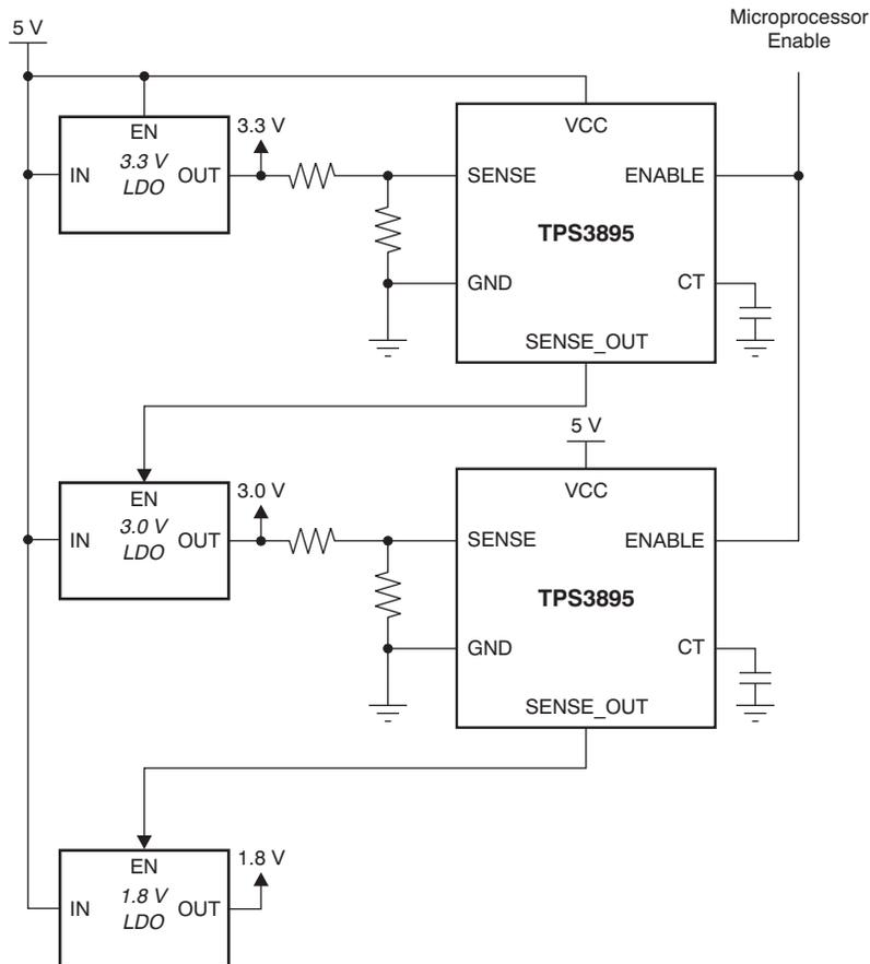
Figure 26. Voltage Sequencing (5 V → 3.3 V → 3.0 V → 1.8 V)
