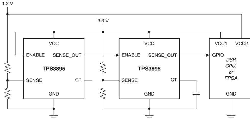
Figure 24. Multiple Voltage Monitoring Using the Enable Pin
