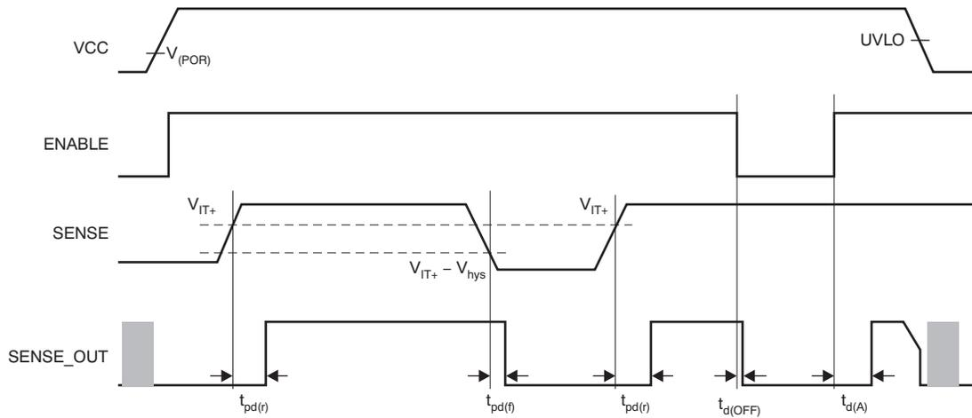
Figure 1. TPS3895A/TPS3897A Timing
