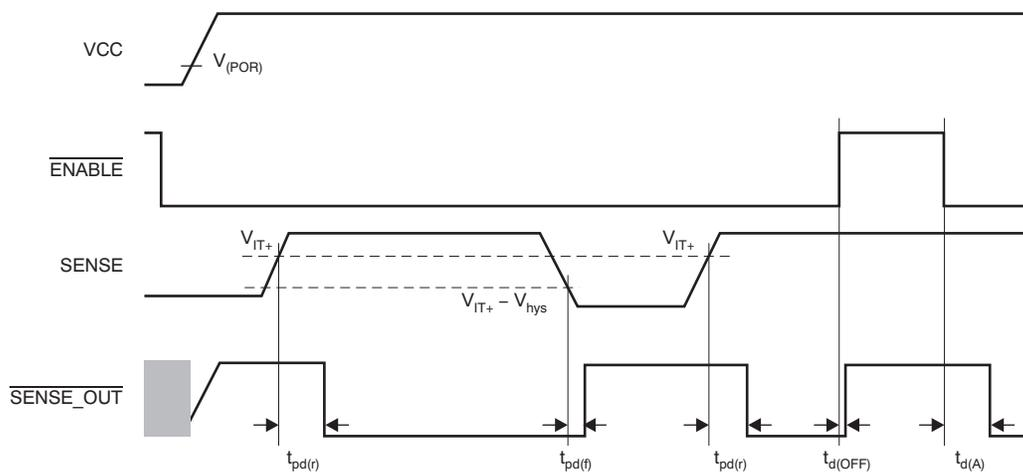
Figure 3. TPS3896A/TPS3898A Timing
