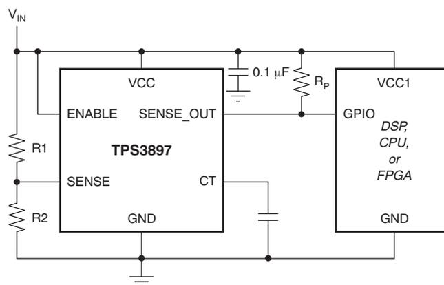
Figure 23. Using TPS3897 to Monitor User-Defined Threshold Voltage
