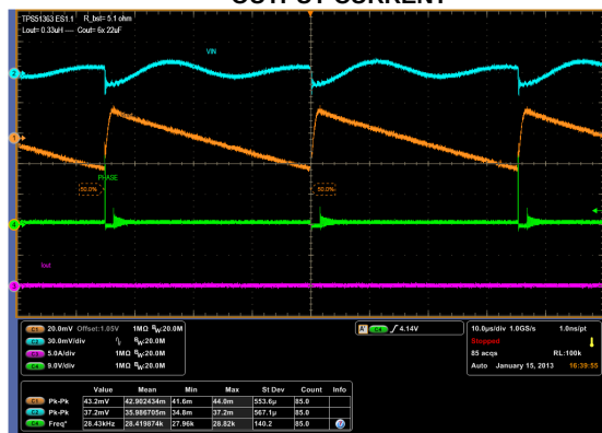
Figure 19. f = 800\text{kHz} , V_{IN} = 20\text{V} , I_{OUT} = 0.1\text{A}
