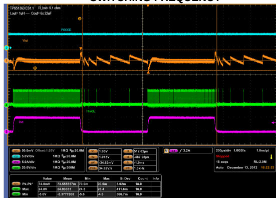
Figure 21. f = 400\text{kHz} , V_{IN} = 20\text{V} , I_{OUT} = 0-5\text{A}
