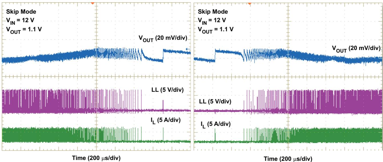
Figure 27. CCM to DCM Transition Waveforms
