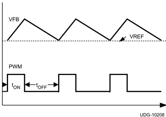
**Figure 36. On-Time Control Without Ramp Compensation**
