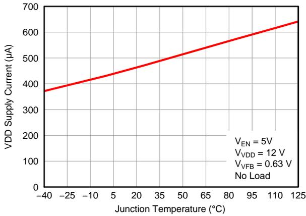
Figure 3. VDD Supply Current vs. Junction Temperature
