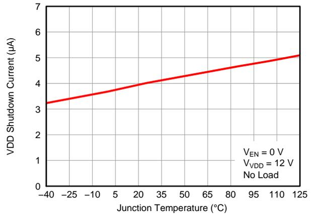
Figure 4. VDD Shutdown Current vs. Junction Temperature
