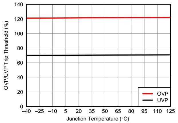
Figure 6. OVP/UVP Trip Threshold vs. Junction Temperature
