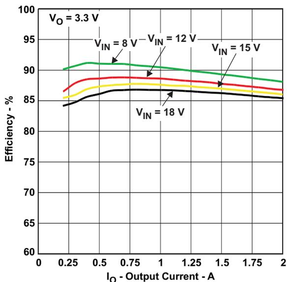
Figure 14. TPS54233 Efficiency
