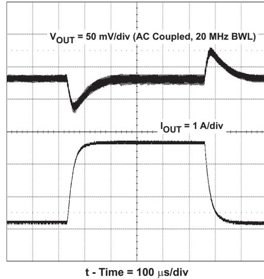
Figure 17. Transient Response,  $I_O$  Step 1.25 to 3.75 A.
