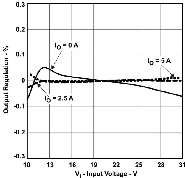
Figure 14. Output Regulation % vs. Input Voltage
