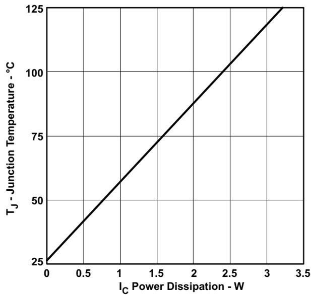
Figure 18. TPS5450 Power Dissipation vs Junction Temperature.
