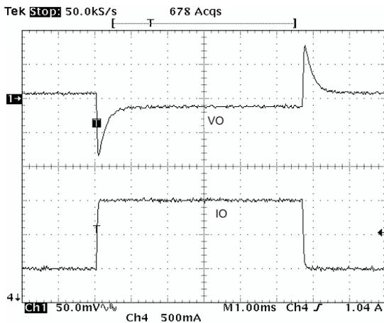
Figure 52. Load Transmit
