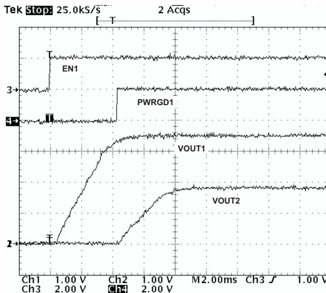
Figure 33. Sequential Start-Up Using EN and PWRGD
