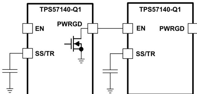
Figure 32. Schematic for Sequential Start-Up Sequence
