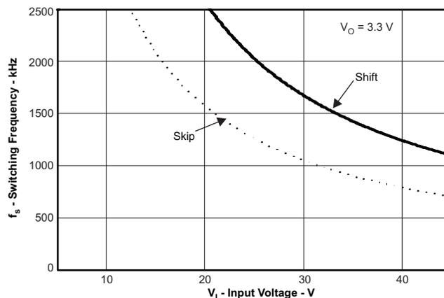
**Figure 42. Maximum Switching Frequency versus Input Voltage**
