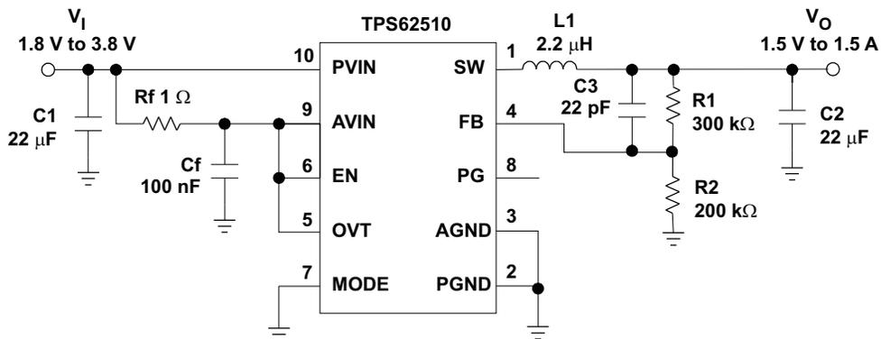
Figure 23. Adjustable Version Programmed to 1.5 V
