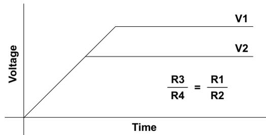
Figure 20. Simultaneous Tracking of V2 and V1
