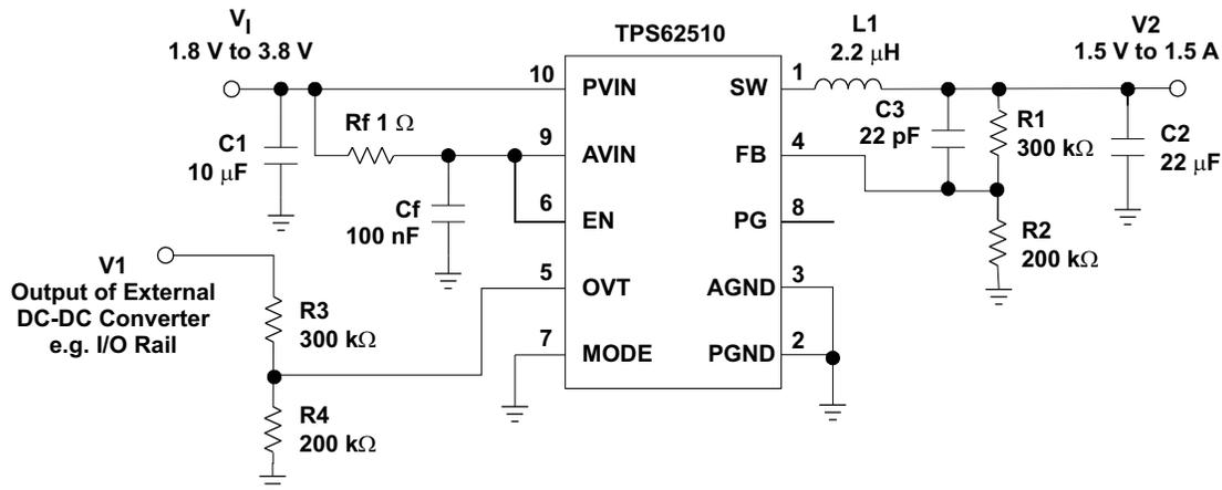
Figure 18. Output Voltage Tracking, V2 Tracks V1
