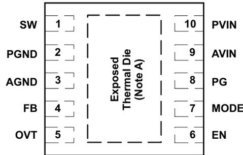
A. The exposed Thermal Die is connected to AGND.
