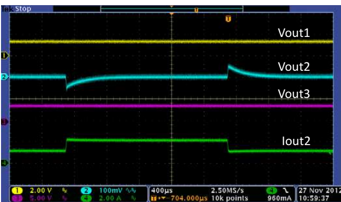
Figure 23. Transient Response Buck2@1.8V, 1-2A Step, C_o = 47\mu\text{F}
