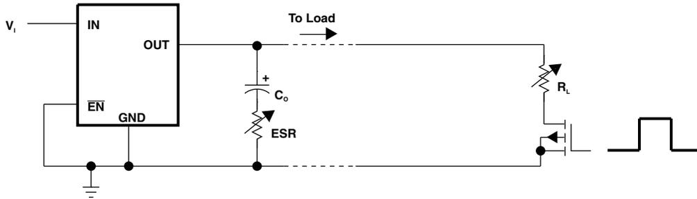
Figure 30. Test Circuit for Typical Regions of Stability
