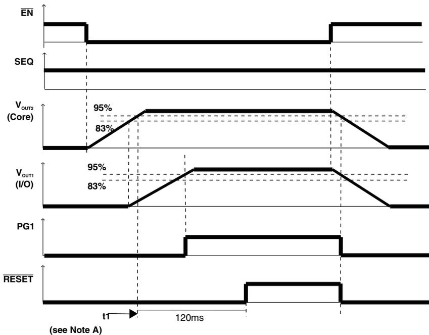
NOTE A:  $t_1$  - Time at which both  $V_{OUT1}$  and  $V_{OUT2}$  are greater than the PG1 thresholds and  $\overline{MR1}$  is logic high.
