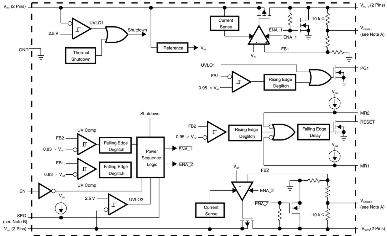
NOTES: A. For most applications,  $V_{SENSE1}$  and  $V_{SENSE2}$  should be externally connected to  $V_{OUT}$  as close as possible to the device. For other implementations, refer to SENSE terminal connection discussion in the Application Information section.
