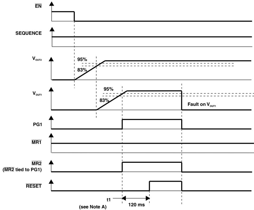
NOTE A:  $t_1$  - Time at which both  $V_{OUT1}$  and  $V_{OUT2}$  are greater than the PG thresholds and  $\overline{MR1}$  is logic high.
