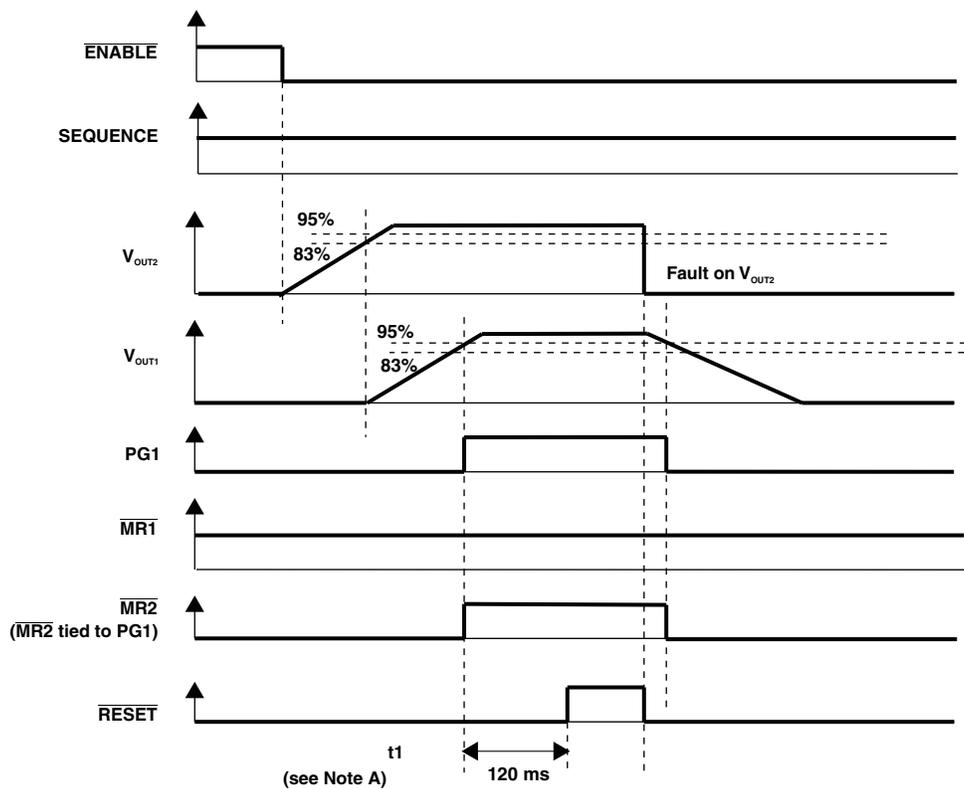
NOTE A: t<sub>1</sub> - Time at which both V<sub>OUT1</sub> and V<sub>OUT2</sub> are greater than the PG thresholds and MR1 is logic high.
