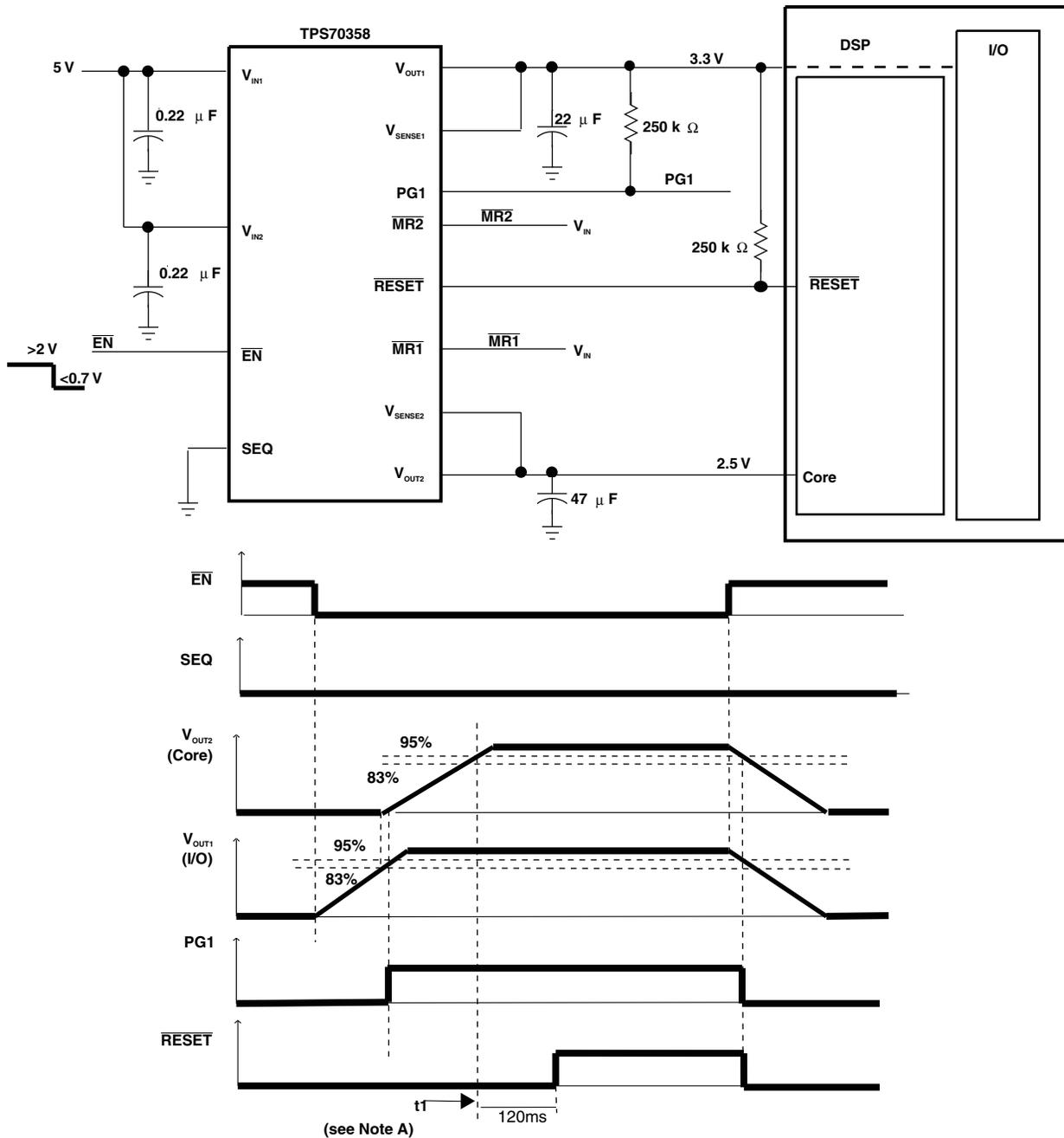
NOTE A:  $t_1$  - Time at which both  $V_{OUT1}$  and  $V_{OUT2}$  are greater than the PG1 thresholds and  $\overline{MR1}$  is logic high.
