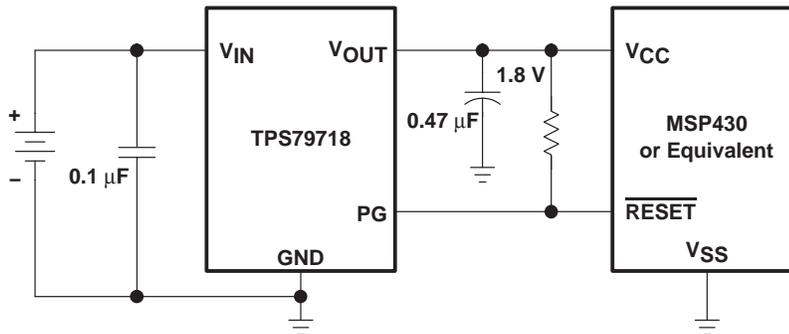
Figure 15. MSP430 Microcontroller Powered by the TPS79718 Regulator
