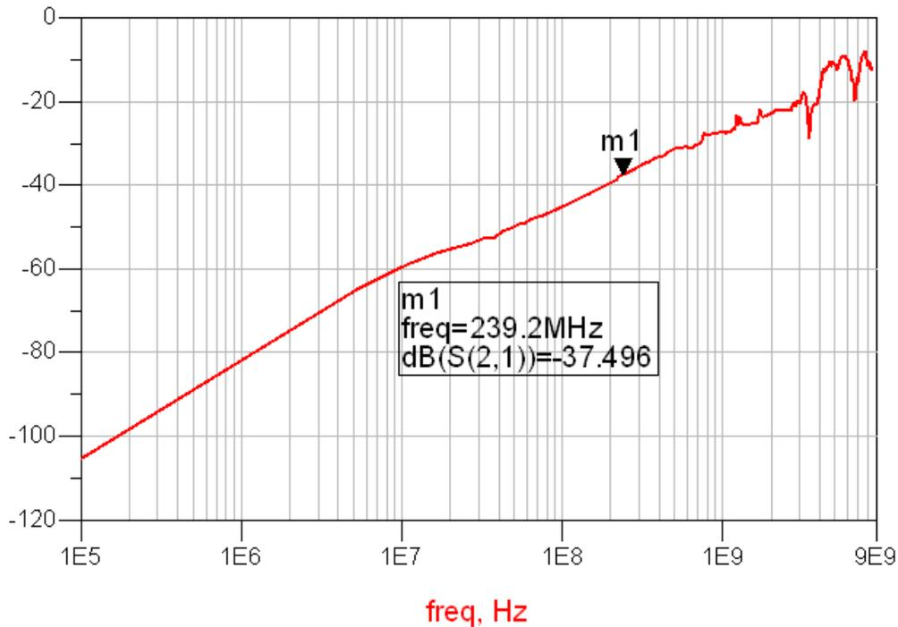
Figure 22. Cross talk vs. Frequency for USB Path
