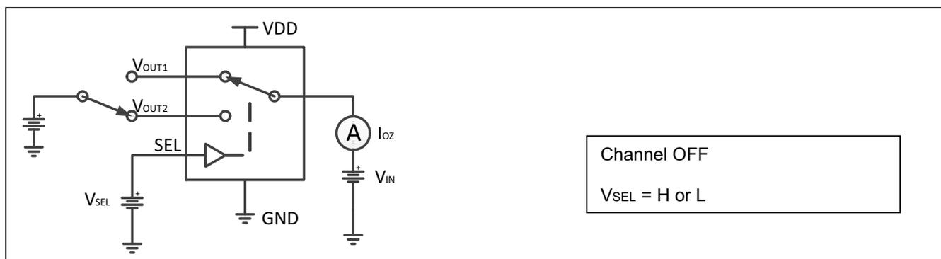
Figure 3. OFF Leakage Current ( $I_{OZ}$ )
