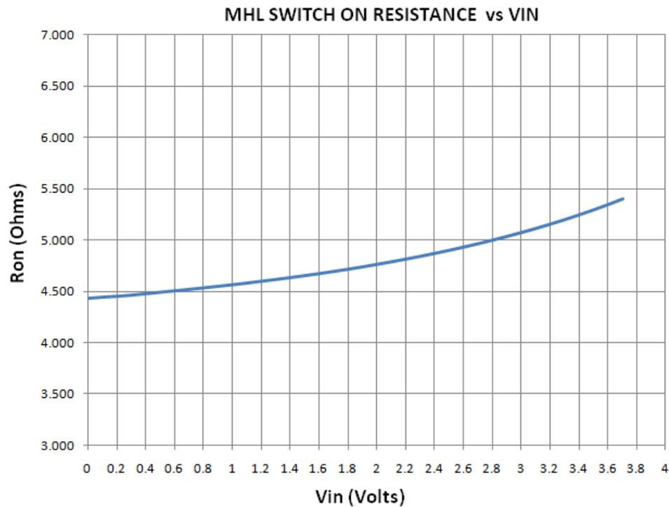
Figure 15. ON-Resistance vs. VI for MHL Switch
