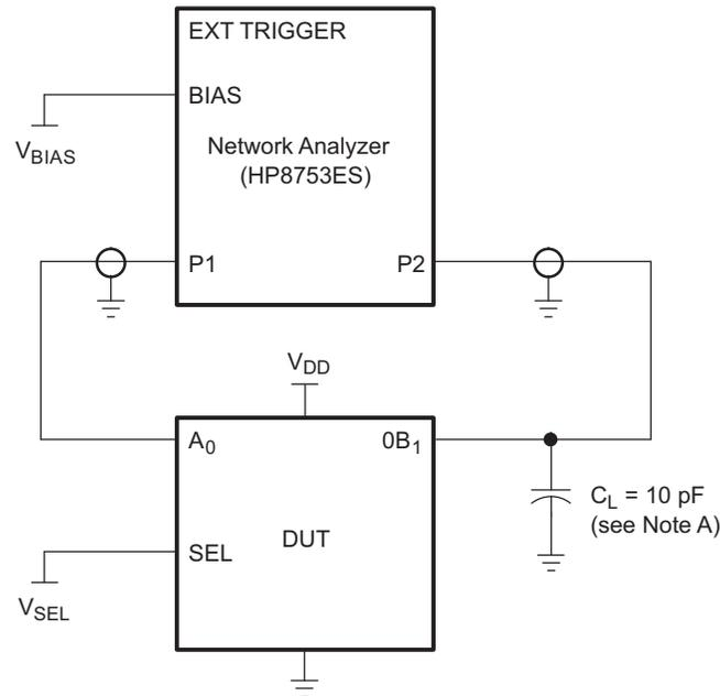
**Figure 6. Test Circuit for Frequency Response (BW)**
