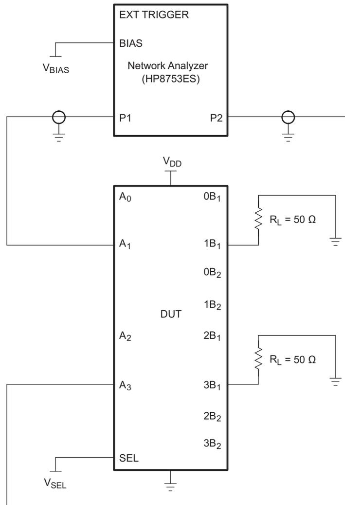
Figure 7. Test Circuit for Crosstalk ( $X_{TALK}$ )
