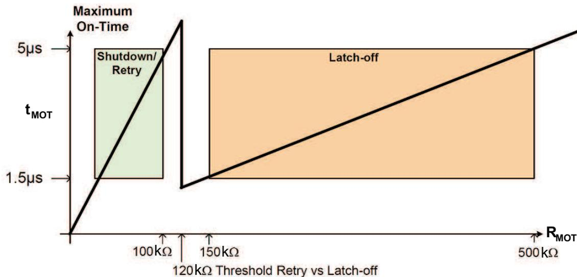
Figure 33. Programming MOT and Overload Fault Response
