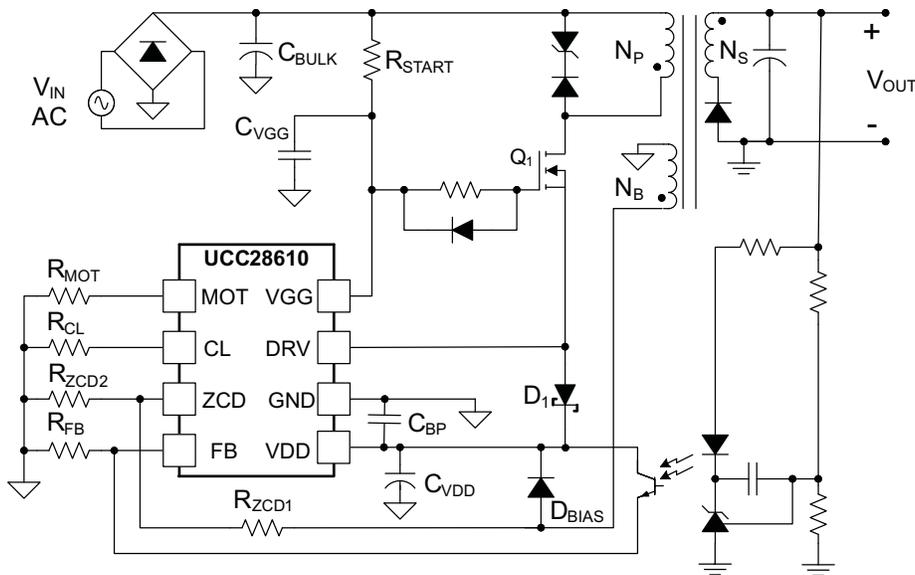
**Figure 1. Recommended Operating Conditions Application**
