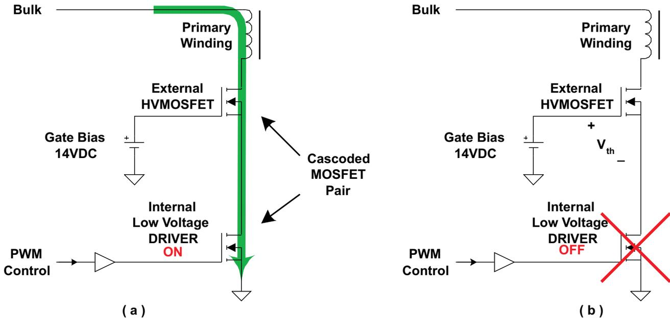
Figure 21. Cascoded Architecture
