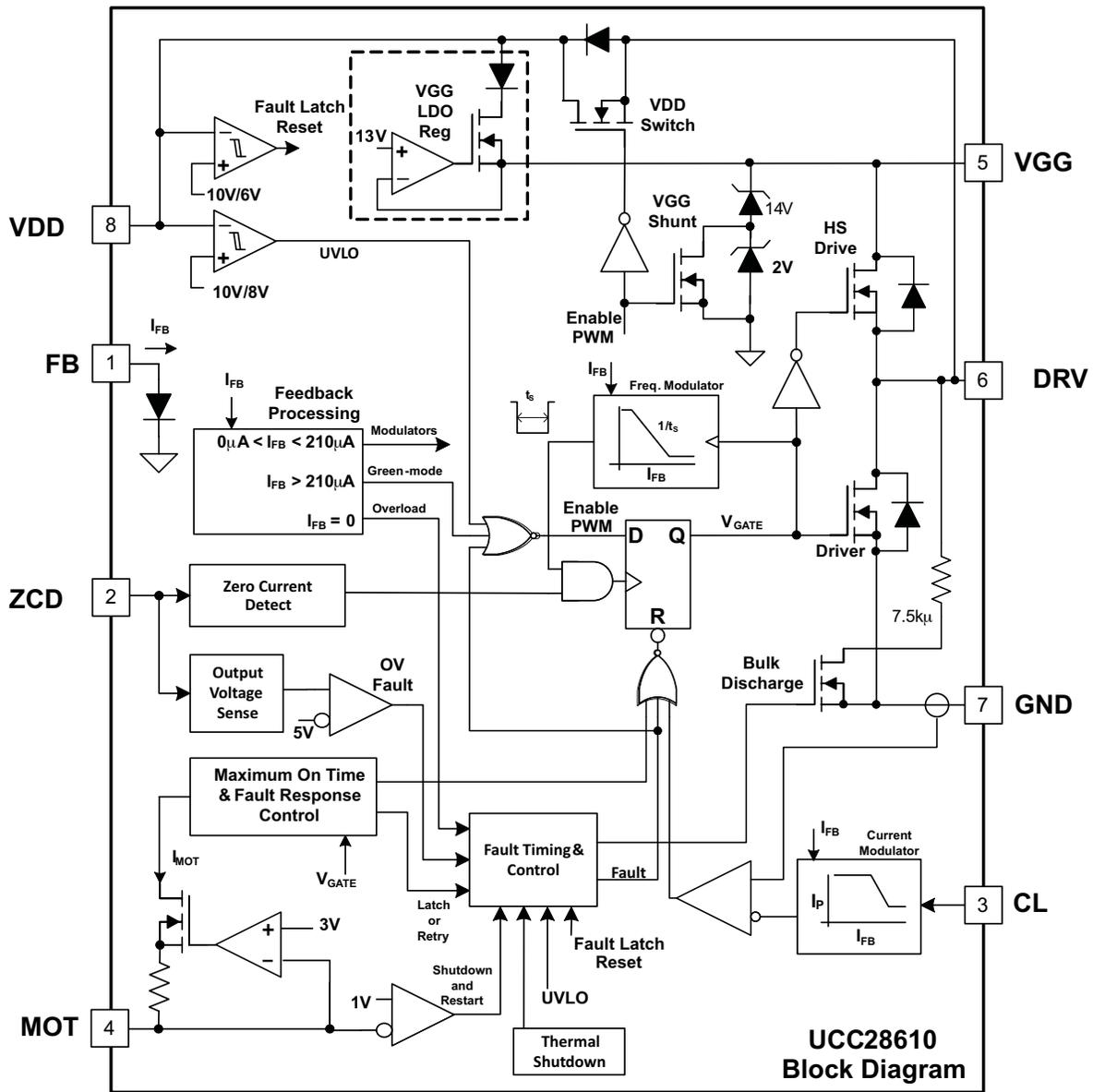
Figure 19. Simplified Block Diagram
