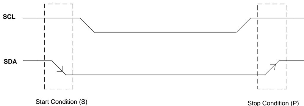
**Figure 1. I<sup>2</sup>C Start and Stop Condition**
