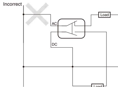
Do not design a circuit where voltage is imposed between contacts, otherwise contact weld may result.
