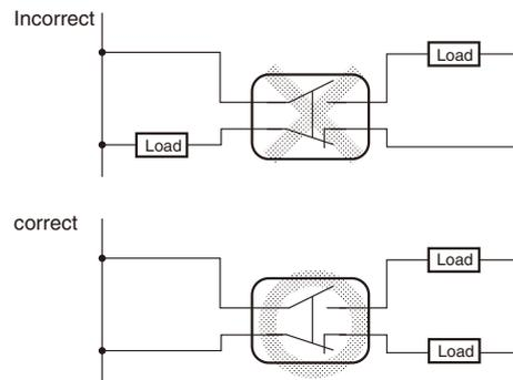
Connect the load to the same polarity.
