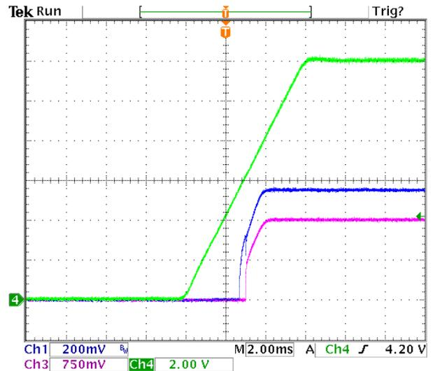
Figure 8. Typical Start-Up with application of Vin (Vo = 0.6Vdc, Io = 20A). Ch1 – Vout, Ch2 – Iout, Ch3 – Iout, Ch4 – Vin.
