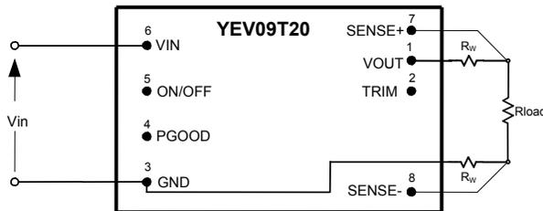
Figure 21. Remote Sense Circuit Configuration
