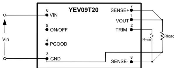
Figure 19. Programming Output Voltage With A Resistor
