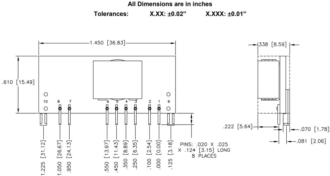
**Figure 23. Mechanical Drawing**
