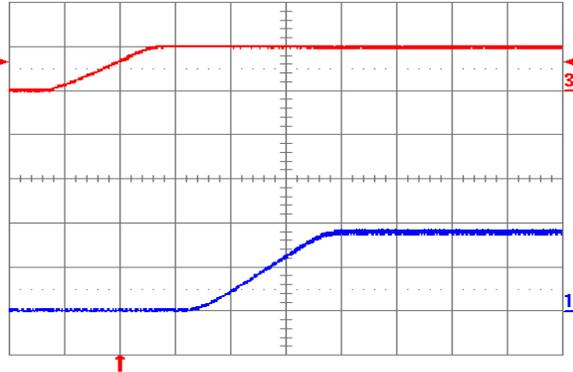
**Fig. 1.8V.5:** Turn-on transient for  $V_{out} = 1.8\text{ V}$  with application of  $V_{in}$  at full rated load current (resistive) and  $47\text{ }\mu\text{F}$  external capacitance at  $V_{in} = 5\text{ V}$ . Top trace:  $V_{in}$  ( $5\text{ V/div.}$ ); Bottom trace: output voltage ( $1\text{ V/div.}$ ); Time scale:  $2\text{ ms/div.}$
