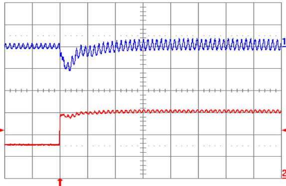
**Fig. 1.2V.7:** Output voltage response for  $V_{out} = 1.2\text{ V}$  to positive load current step change from  $2.5\text{ A}$  to  $5\text{ A}$  with slew rate of  $5\text{ A}/\mu\text{s}$  at  $V_{in} = 5\text{ V}$ . Top trace: output voltage ( $100\text{ mV/div.}$ ); Bottom trace: load current ( $2\text{ A/div.}$ ).  $C_o = 47\text{ }\mu\text{F}$  ceramic +  $1\text{ }\mu\text{F}$  ceramic. Time scale:  $20\text{ }\mu\text{s/div.}$
