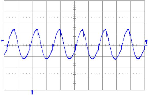
**Fig. 1.5V.6:** Output voltage ripple ( $20\text{ mV/div.}$ ) at full rated load current into a resistive load with external capacitance  $10\text{ }\mu\text{F}$  ceramic +  $1\text{ }\mu\text{F}$  ceramic and  $V_{in} = 5\text{ V}$  for  $V_{out} = 1.5\text{ V}$ . Time scale:  $2\text{ }\mu\text{s/div.}$
