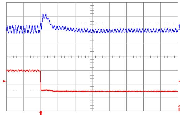
**Fig. 1.8V.8:** Output voltage response for  $V_{out} = 1.8\text{ V}$  to negative load current step change from  $5\text{ A}$  to  $2.5\text{ A}$  with slew rate of  $-5\text{ A}/\mu\text{s}$  at  $V_{in} = 5\text{ V}$ . Top trace: output voltage ( $100\text{ mV/div.}$ ); Bottom trace: load current ( $2\text{ A/div.}$ ).  $C_o = 47\text{ }\mu\text{F}$  ceramic +  $1\text{ }\mu\text{F}$  ceramic. Time scale:  $20\text{ }\mu\text{s/div.}$
