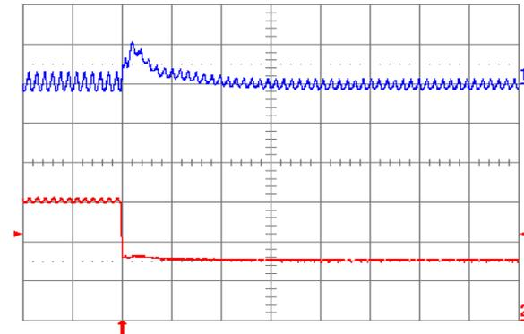
**Fig. 1.2V.8:** Output voltage response for  $V_{out} = 1.2\text{ V}$  to negative load current step change from  $5\text{ A}$  to  $2.5\text{ A}$  with slew rate of  $-5\text{ A}/\mu\text{s}$  at  $V_{in} = 5\text{ V}$ . Top trace: output voltage ( $100\text{ mV/div.}$ ); Bottom trace: load current ( $2\text{ A/div.}$ ).  $C_o = 47\text{ }\mu\text{F}$  ceramic +  $1\text{ }\mu\text{F}$  ceramic. Time scale:  $20\text{ }\mu\text{s/div.}$
