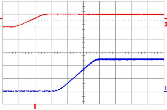
**Fig. 2.5V.4:** Turn-on transient for  $V_{out} = 2.5$  V with application of  $V_{in}$  at full rated load current (resistive) and 47  $\mu$ F external capacitance at  $V_{in} = 5$  V. Top trace:  $V_{in}$  (5 V/div.); Bottom trace: output voltage (1V/div.); Time scale: 2 ms/div.
