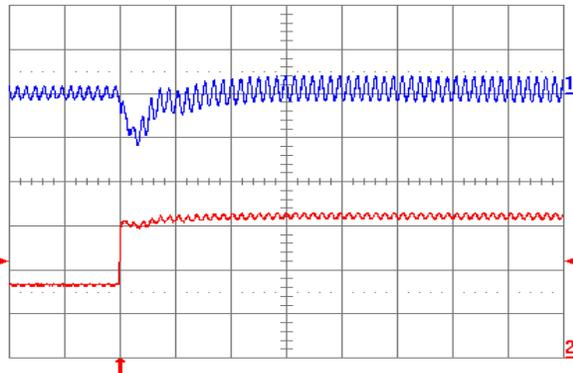
**Fig. 1.5V.7:** Output voltage response for  $V_{out} = 1.5\text{ V}$  to positive load current step change from  $2.5\text{ A}$  to  $5\text{ A}$  with slew rate of  $5\text{ A}/\mu\text{s}$  at  $V_{in} = 5\text{ V}$ . Top trace: output voltage ( $100\text{ mV/div.}$ ); Bottom trace: load current ( $2\text{ A/div.}$ ).  $C_o = 47\text{ }\mu\text{F}$  ceramic +  $1\text{ }\mu\text{F}$  ceramic. Time scale:  $20\text{ }\mu\text{s/div.}$
