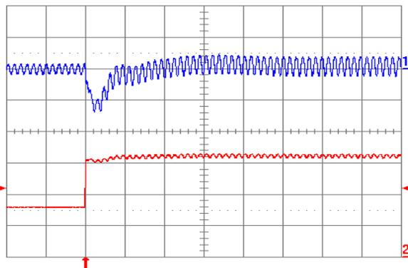
**Fig. 2.5V.7:** Output voltage response for  $V_{out} = 2.5$  V to positive load current step change from 2.5 A to 5 A with slew rate of 5 A/ $\mu$ s at  $V_{in} = 5$  V. Top trace: output voltage (100 mV/div.); Bottom trace: load current (2 A/div.).  $C_o = 47$   $\mu$ F ceramic + 1  $\mu$ F ceramic. Time scale: 20  $\mu$ s/div.
