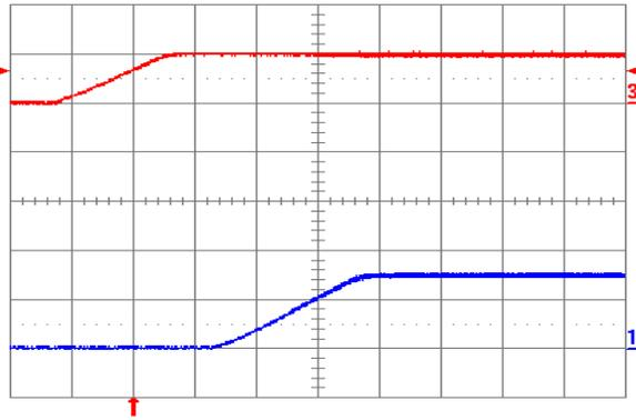
**Fig. 1.5V.5:** Turn-on transient for  $V_{out} = 1.5\text{ V}$  with application of  $V_{in}$  at full rated load current (resistive) and  $47\text{ }\mu\text{F}$  external capacitance at  $V_{in} = 5\text{ V}$ . Top trace:  $V_{in}$  ( $5\text{ V/div.}$ ); Bottom trace: output voltage ( $1\text{ V/div.}$ ); Time scale:  $2\text{ ms/div.}$
