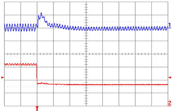
**Fig. 1.5V.8:** Output voltage response for  $V_{out} = 1.5\text{ V}$  to negative load current step change from  $5\text{ A}$  to  $2.5\text{ A}$  with slew rate of  $-5\text{ A}/\mu\text{s}$  at  $V_{in} = 5\text{ V}$ . Top trace: output voltage ( $100\text{ mV/div.}$ ); Bottom trace: load current ( $2\text{ A/div.}$ ).  $C_o = 47\text{ }\mu\text{F}$  ceramic +  $1\text{ }\mu\text{F}$  ceramic. Time scale:  $20\text{ }\mu\text{s/div.}$
