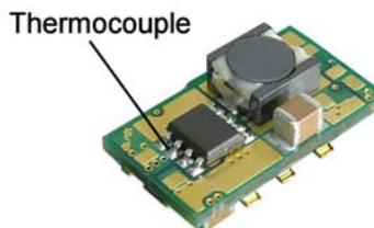
**Fig. C:** Location of the thermocouple for thermal testing.
