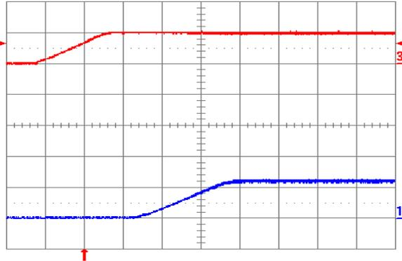
**Fig. 1.2V.5:** Turn-on transient for  $V_{out} = 1.2\text{ V}$  with application of  $V_{in}$  at full rated load current (resistive) and  $47\text{ }\mu\text{F}$  external capacitance at  $V_{in} = 5\text{ V}$ . Top trace:  $V_{in}$  ( $5\text{ V/div.}$ ); Bottom trace: output voltage ( $1\text{ V/div.}$ ); Time scale:  $2\text{ ms/div.}$
