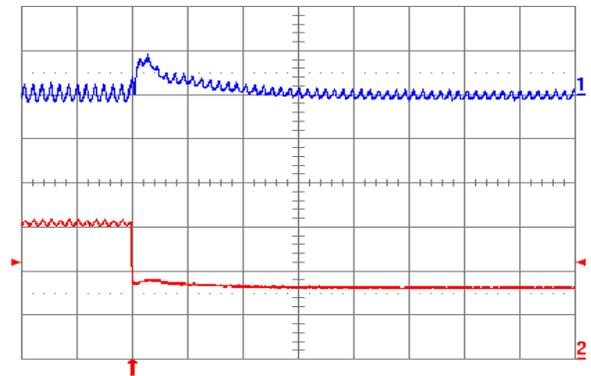
**Fig. 0.7525V.8:** Output voltage response for  $V_{out} = 0.7525$  V to negative load current step change from 5 A to 2.5 A with slew rate of  $-5 \text{ A}/\mu\text{s}$  at  $V_{in} = 5$  V. Top trace: output voltage (100 mV/div.); Bottom trace: load current (2 A/div.).  $C_o = 47 \mu\text{F}$  ceramic +  $1 \mu\text{F}$  ceramic. Time scale:  $20 \mu\text{s}/\text{div}$ .
