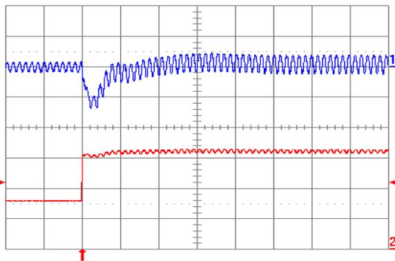
**Fig. 2.5V.7:** Output voltage response for  $V_{out} = 2.5\text{ V}$  to positive load current step change from 2.5 A to 5 A with slew rate of  $5\text{ A}/\mu\text{s}$  at  $V_{in} = 5\text{ V}$ . Top trace: output voltage (100 mV/div.); Bottom trace: load current (2 A/div.).  $C_o = 47\ \mu\text{F}$  ceramic +  $1\ \mu\text{F}$  ceramic. Time scale: 20  $\mu\text{s}$ /div.
