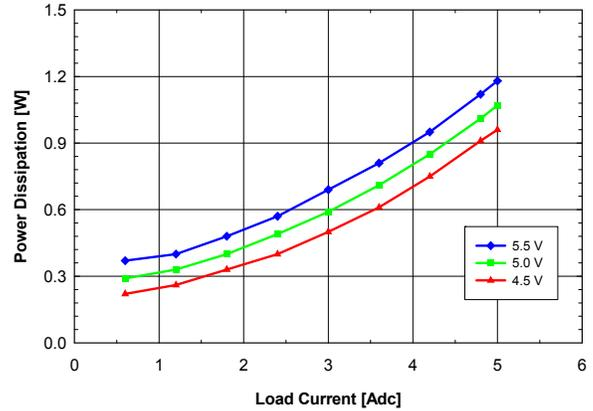
**Fig. 3.3V.4:** Power Loss vs. load current and input voltage for  $V_{out} = 3.3\text{ V}$  converter mounted vertically with air flowing from pin 5 to pin 1 at a rate of 200 LFM (1 m/s) and  $T_a = 25\text{ }^{\circ}\text{C}$ .
