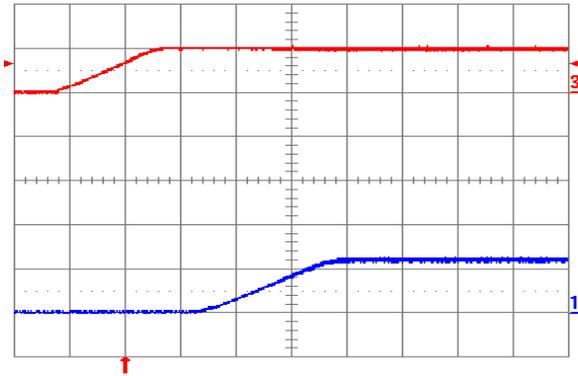
Fig. 1.2V.5: Turn-on transient for  $V_{out} = 1.2\text{ V}$  with application of  $V_{in}$  at full rated load current (resistive) and  $47\text{ }\mu\text{F}$  external capacitance at  $V_{in} = 5\text{ V}$ . Top trace:  $V_{in}$  (5 V/div.); Bottom trace: output voltage (1 V/div.); Time scale: 2 ms/div.
