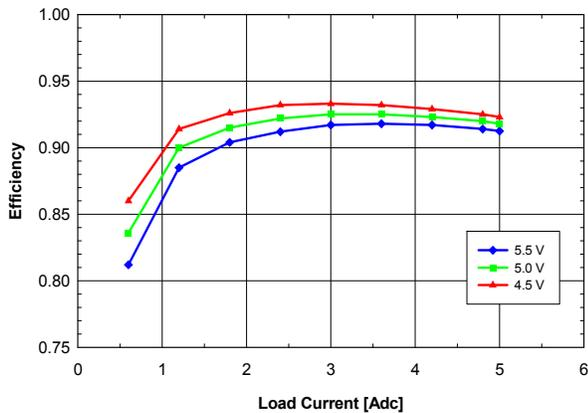
**Fig. 2.5V.3:** Efficiency vs. load current and input voltage for  $V_{out} = 2.5\text{ V}$  converter mounted vertically with air flowing from pin 5 to pin 1 at a rate of 200 LFM (1 m/s) and  $T_a = 25\text{ }^{\circ}\text{C}$ .
