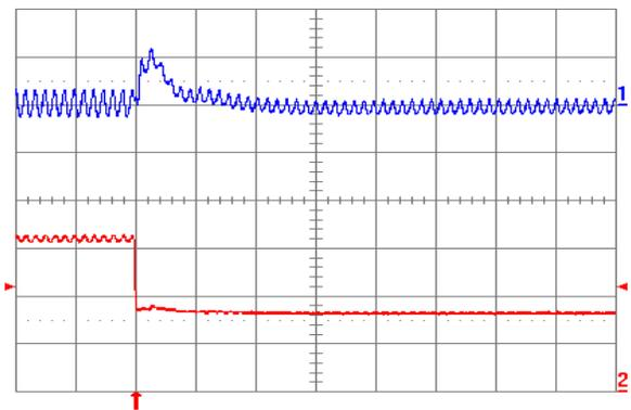
**Fig. 1.5V.8:** Output voltage response for  $V_{out} = 1.5\text{ V}$  to negative load current step change from 5 A to 2.5 A with slew rate of  $-5\text{ A}/\mu\text{s}$  at  $V_{in} = 5\text{ V}$ . Top trace: output voltage (100 mV/div.); Bottom trace: load current (2 A/div.).  $C_o = 47\ \mu\text{F}$  ceramic +  $1\ \mu\text{F}$  ceramic. Time scale: 20  $\mu\text{s}$ /div.
