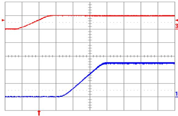
**Fig. 2.5V.4:** Turn-on transient for  $V_{out} = 2.5\text{ V}$  with application of  $V_{in}$  at full rated load current (resistive) and  $47\ \mu\text{F}$  external capacitance at  $V_{in} = 5\text{ V}$ . Top trace:  $V_{in}$  (5 V/div.); Bottom trace: output voltage (1V/div.); Time scale: 2 ms/div.
