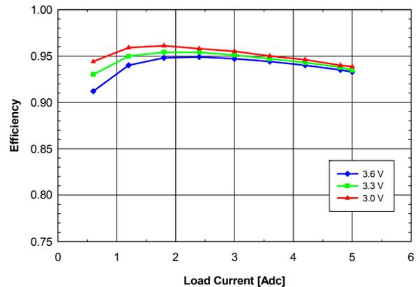
**Fig. 2.5V.4:** Efficiency vs. load current and input voltage for  $V_{out} = 2.5\text{ V}$  converter mounted vertically with air flowing from pin 5 to pin 1 at a rate of 200 LFM (1 m/s) and  $T_a = 25\text{ }^{\circ}\text{C}$ .
