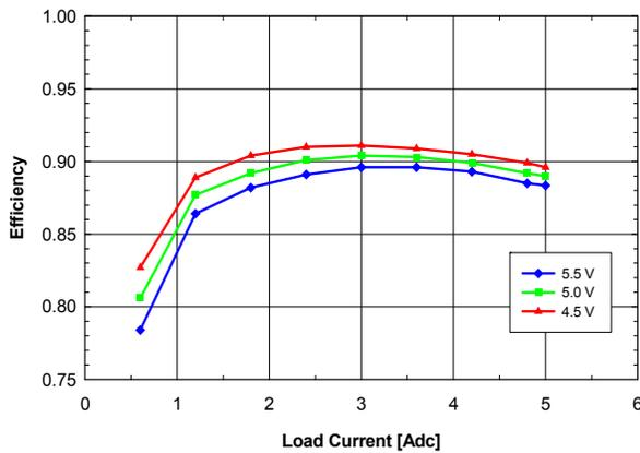
**Fig. 1.8V.3:** Efficiency vs. load current and input voltage for  $V_{out} = 1.8\text{ V}$  converter mounted vertically with air flowing from pin 5 to pin 1 at a rate of 200 LFM (1 m/s) and  $T_a = 25\text{ }^{\circ}\text{C}$ .
