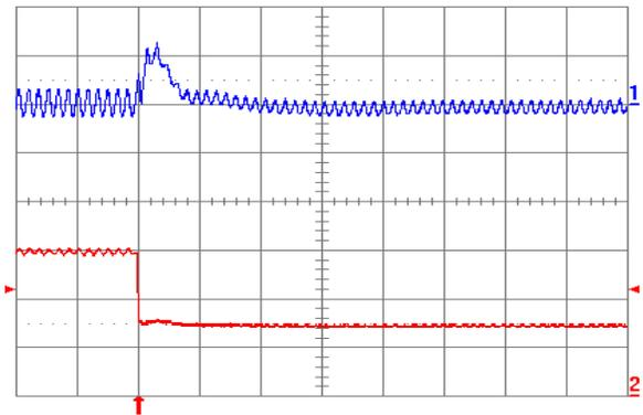
Fig. 1.8V.8: Output voltage response for  $V_{out} = 1.8\text{ V}$  to negative load current step change from 5 A to 2.5 A with slew rate of  $-5\text{ A}/\mu\text{s}$  at  $V_{in} = 5\text{ V}$ . Top trace: output voltage (100 mV/div.); Bottom trace: load current (2 A/div.).  $C_o = 47\text{ }\mu\text{F}$  ceramic +  $1\text{ }\mu\text{F}$  ceramic. Time scale: 20  $\mu\text{s}$ /div.
