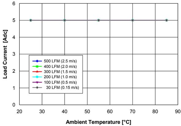
**Fig. 2.5V.1:** Available load current vs. ambient temperature and airflow rates for  $V_{out} = 2.5\text{ V}$  converter mounted vertically with  $V_{in} = 5\text{ V}$ , air flowing from pin 5 to pin 1, and maximum MOSFET temperature  $\leq 120\text{ }^{\circ}\text{C}$ .
