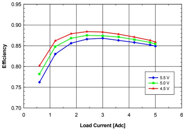
**Fig. 1.2V.3: Efficiency vs. load current and input voltage for  $V_{out} = 1.2\text{ V}$  converter mounted vertically with air flowing from pin 5 to pin 1 at a rate of 200 LFM (1 m/s) and  $T_a = 25\text{ }^{\circ}\text{C}$ .**
