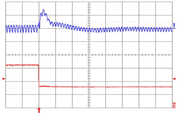
Fig. 3.3V.8: Output voltage response for  $V_{out} = 3.3\text{ V}$  to negative load current step change from 5 A to 2.5 A with slew rate of  $-5\text{ A}/\mu\text{s}$  at  $V_{in} = 5\text{ V}$ . Top trace: output voltage (100 mV/div.); Bottom trace: load current (2 A/div.).  $C_o = 47\text{ }\mu\text{F}$  ceramic +  $1\text{ }\mu\text{F}$  ceramic. Time scale: 20  $\mu\text{s}$ /div.
