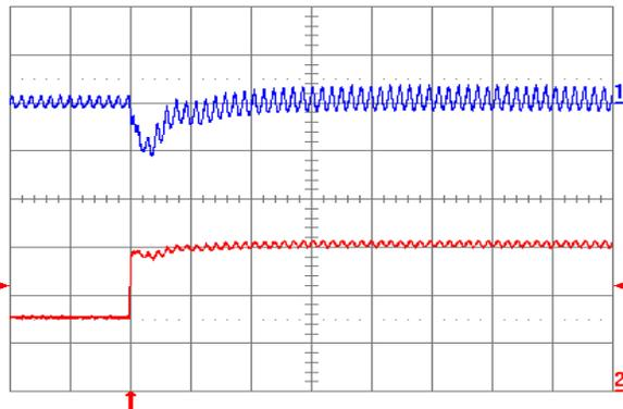
Fig. 1.2V.6: Output voltage response for  $V_{out} = 1.2\text{ V}$  to positive load current step change from 2.5 A to 5 A with slew rate of  $5\text{ A}/\mu\text{s}$  at  $V_{in} = 5\text{ V}$ . Top trace: output voltage (100 mV/div.); Bottom trace: load current (2 A/div.).  $C_o = 47\text{ }\mu\text{F}$  ceramic +  $1\text{ }\mu\text{F}$  ceramic. Time scale: 20  $\mu\text{s}$ /div.
