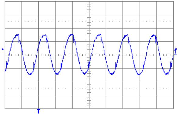
**Fig. 2.0V.6:** Output voltage ripple (20 mV/div.) at full rated load current into a resistive load with external capacitance  $10 \mu\text{F}$  ceramic +  $1 \mu\text{F}$  ceramic and  $V_{in} = 5$  V for  $V_{out} = 2.0$  V. Time scale: 2  $\mu\text{s}$ /div.
