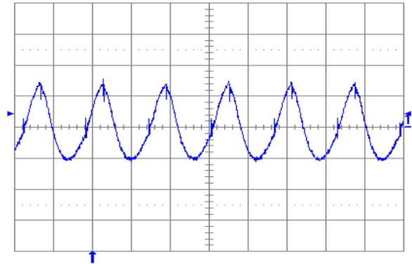
Fig. 1.2V.6: Output voltage ripple (20 mV/div.) at full rated load current into a resistive load with external capacitance  $10\text{ }\mu\text{F}$  ceramic +  $1\text{ }\mu\text{F}$  ceramic and  $V_{in} = 5\text{ V}$  for  $V_{out} = 1.2\text{ V}$ . Time scale: 2  $\mu\text{s}$ /div.
