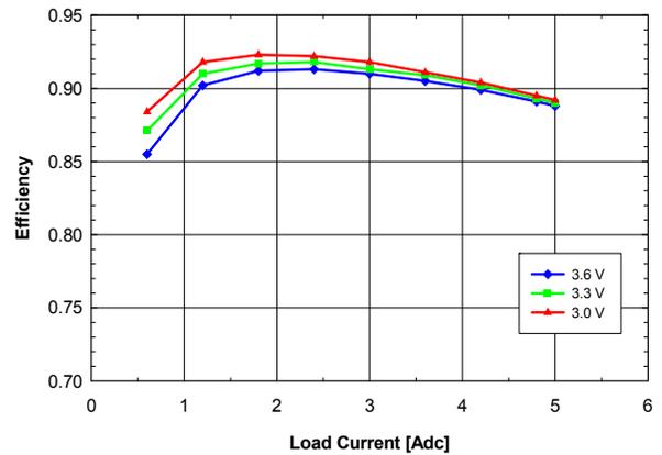
**Fig. 1.5V.4:** Efficiency vs. load current and input voltage for  $V_{out} = 1.5\text{ V}$  converter mounted vertically with air flowing from pin 5 to pin 1 at a rate of 200 LFM (1 m/s) and  $T_a = 25\text{ }^{\circ}\text{C}$ .
