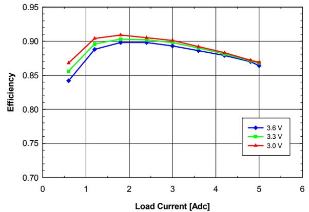
**Fig. 1.2V.4: Efficiency vs. load current and input voltage for  $V_{out} = 1.2\text{ V}$  converter mounted vertically with air flowing from pin 5 to pin 1 at a rate of 200 LFM (1m/s) and  $T_a = 25\text{ }^{\circ}\text{C}$ .**
