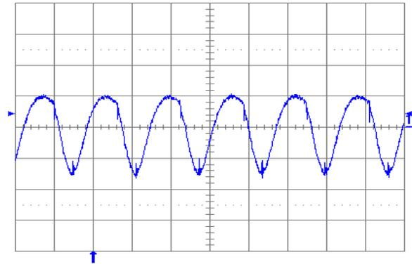
Fig. 3.3V.6: Output voltage ripple (20 mV/div.) at full rated load current into a resistive load with external capacitance  $10\text{ }\mu\text{F}$  ceramic +  $1\text{ }\mu\text{F}$  ceramic and  $V_{in} = 5\text{ V}$  for  $V_{out} = 3.3\text{ V}$ . Time scale: 2  $\mu\text{s}$ /div.
