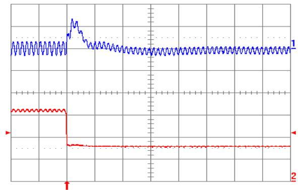
**Fig. 2.5V.8:** Output voltage response for  $V_{out} = 2.5\text{ V}$  to negative load current step change from 5 A to 2.5 A with slew rate of  $-5\text{ A}/\mu\text{s}$  at  $V_{in} = 5\text{ V}$ . Top trace: output voltage (100 mV/div.); Bottom trace: load current (2 A/div.).  $C_o = 47\ \mu\text{F}$  ceramic +  $1\ \mu\text{F}$  ceramic. Time scale: 20  $\mu\text{s}$ /div.
