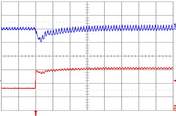
**Fig. 0.7525V.7:** Output voltage response for  $V_{out} = 0.7525$  V to positive load current step change from 2.5 A to 5 A with slew rate of  $5 \text{ A}/\mu\text{s}$  at  $V_{in} = 5$  V. Top trace: output voltage (100 mV/div.); Bottom trace: load current (2 A/div.).  $C_o = 47 \mu\text{F}$  ceramic +  $1 \mu\text{F}$  ceramic. Time scale:  $20 \mu\text{s}/\text{div}$ .
