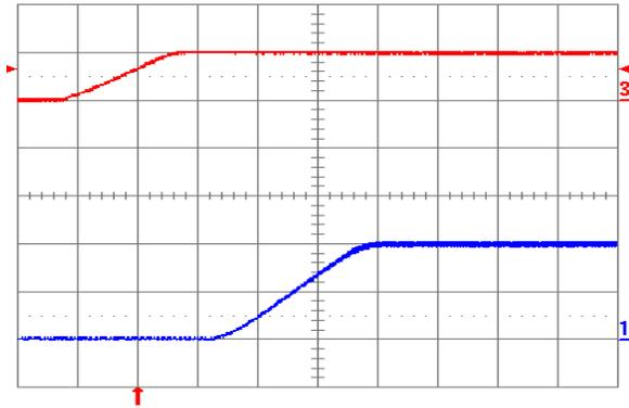
**Fig. 2.0V.5:** Turn-on transient for  $V_{out} = 2.0$  V with application of  $V_{in}$  at full rated load current (resistive) and  $47 \mu\text{F}$  external capacitance at  $V_{in} = 5$  V. Top trace:  $V_{in}$  (5 V/div.); Bottom trace: output voltage (1 V/div.); Time scale: 2 ms/div.
