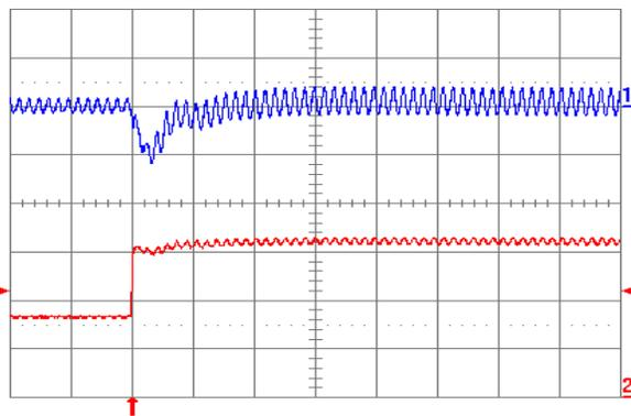
**Fig. 1.5V.7:** Output voltage response for  $V_{out} = 1.5\text{ V}$  to positive load current step change from 2.5 A to 5 A with slew rate of  $5\text{ A}/\mu\text{s}$  at  $V_{in} = 5\text{ V}$ . Top trace: output voltage (100 mV/div.); Bottom trace: load current (2 A/div.).  $C_o = 47\ \mu\text{F}$  ceramic +  $1\ \mu\text{F}$  ceramic. Time scale: 20  $\mu\text{s}$ /div.
