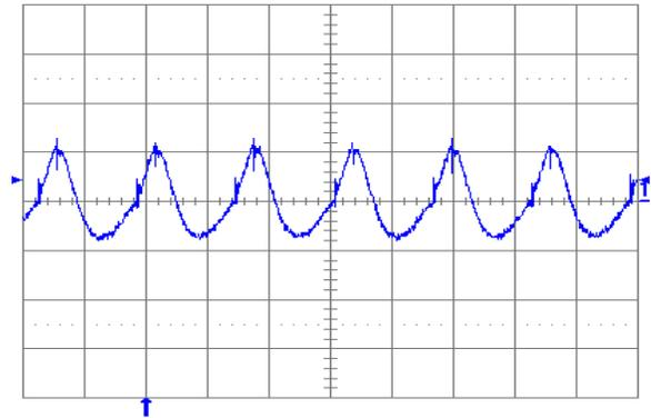
**Fig. 0.7525V.5:** Output voltage ripple (20 mV/div.) at full rated load current into a resistive load with external capacitance  $10 \mu\text{F}$  ceramic +  $1 \mu\text{F}$  ceramic and  $V_{in} = 5$  V for  $V_{out} = 0.7525$  V. Time scale:  $2 \mu\text{s}/\text{div}$ .
