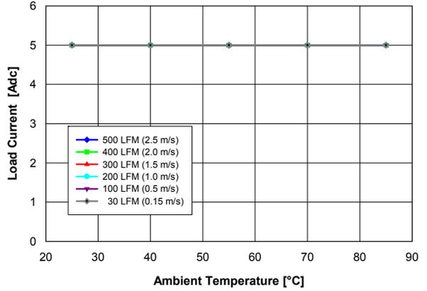
**Fig. 3.3V.2:** Available load current vs. ambient temperature and airflow rates for  $V_{out} = 3.3\text{ V}$  converter mounted horizontally with  $V_{in} = 5\text{ V}$ , air flowing from pin 5 to pin 1, and maximum MOSFET temperature  $\leq 120\text{ }^{\circ}\text{C}$ .
