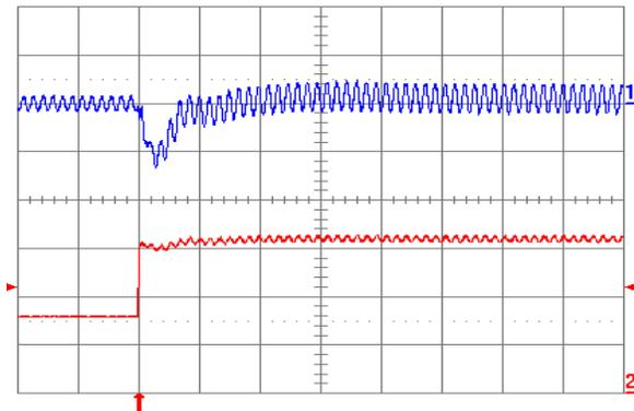
**Fig. 2.0V.7:** Output voltage response for  $V_{out} = 2.0$  V to positive load current step change from 2.5 A to 5 A with slew rate of  $5 \text{ A}/\mu\text{s}$  at  $V_{in} = 5$  V. Top trace: output voltage (100 mV/div.); Bottom trace: load current (2 A/div.).  $C_o = 47 \mu\text{F}$  ceramic +  $1 \mu\text{F}$  ceramic. Time scale: 20  $\mu\text{s}$ /div.
