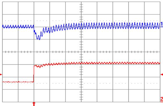
Fig. 1.0V.7: Output voltage response for  $V_{out} = 1.0$  V to positive load current step change from 2.5 A to 5 A with slew rate of  $5 \text{ A}/\mu\text{s}$  at  $V_{in} = 5$  V. Top trace: output voltage (100 mV/div.); Bottom trace: load current (2 A/div.).  $C_o = 47 \mu\text{F}$  ceramic +  $1 \mu\text{F}$  ceramic. Time scale: 20  $\mu\text{s}$ /div.
