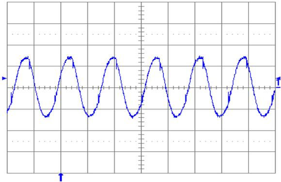
Fig. 1.8V.6: Output voltage ripple (20 mV/div.) at full rated load current into a resistive load with external capacitance  $10\text{ }\mu\text{F}$  ceramic +  $1\text{ }\mu\text{F}$  ceramic and  $V_{in} = 5\text{ V}$  for  $V_{out} = 1.8\text{ V}$ . Time scale: 2  $\mu\text{s}$ /div.
