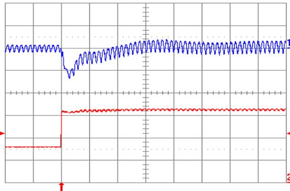
Fig. 3.3V.7: Output voltage response for  $V_{out} = 3.3\text{ V}$  to positive load current step change from 2.5 A to 5 A with slew rate of  $5\text{ A}/\mu\text{s}$  at  $V_{in} = 5\text{ V}$ . Top trace: output voltage (100 mV/div.); Bottom trace: load current (2 A/div.).  $C_o = 47\text{ }\mu\text{F}$  ceramic +  $1\text{ }\mu\text{F}$  ceramic. Time scale: 20  $\mu\text{s}$ /div.
