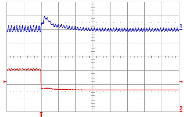
Fig. 1.0V.8: Output voltage response for  $V_{out} = 1.0$  V to negative load current step change from 5 A to 2.5 A with slew rate of  $-5 \text{ A}/\mu\text{s}$  at  $V_{in} = 5$  V. Top trace: output voltage (100 mV/div.); Bottom trace: load current (2 A/div.).  $C_o = 47 \mu\text{F}$  ceramic +  $1 \mu\text{F}$  ceramic. Time scale: 20  $\mu\text{s}$ /div.
