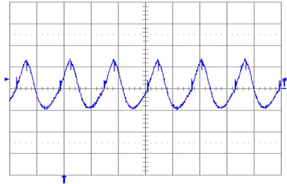
Fig. 1.0V.6: Output voltage ripple (20 mV/div.) at full rated load current into a resistive load with external capacitance  $10 \mu\text{F}$  ceramic +  $1 \mu\text{F}$  ceramic and  $V_{in} = 5$  V for  $V_{out} = 1.0$  V. Time scale: 2  $\mu\text{s}$ /div.
