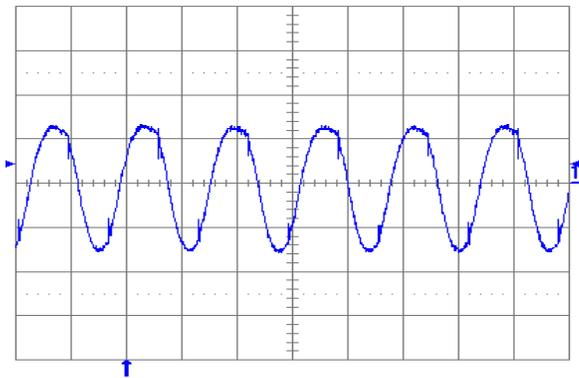
**Fig. 2.5V.5:** Output voltage ripple (20 mV/div.) at full rated load current into a resistive load with external capacitance  $10\ \mu\text{F}$  ceramic +  $1\ \mu\text{F}$  ceramic and  $V_{in} = 5\text{ V}$  for  $V_{out} = 2.5\text{ V}$ . Time scale: 2  $\mu\text{s}$ /div.
