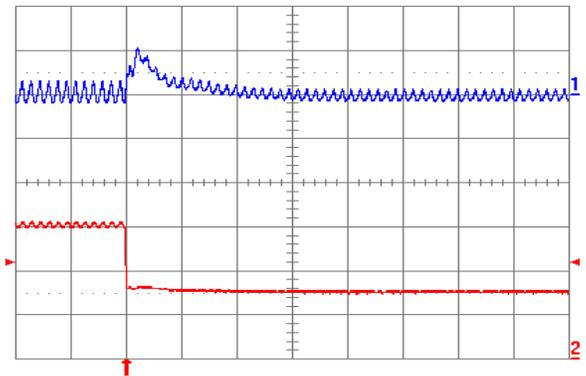
Fig. 1.2V.8: Output voltage response for  $V_{out} = 1.2\text{ V}$  to negative load current step change from 5 A to 2.5 A with slew rate of  $-5\text{ A}/\mu\text{s}$  at  $V_{in} = 5\text{ V}$ . Top trace: output voltage (100 mV/div.); Bottom trace: load current (2 A/div.).  $C_o = 47\text{ }\mu\text{F}$  ceramic +  $1\text{ }\mu\text{F}$  ceramic. Time scale: 20  $\mu\text{s}$ /div.
