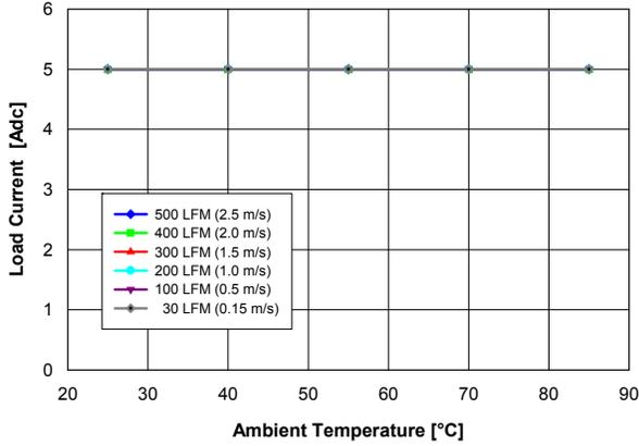
**Fig. 3.3V.1:** Available load current vs. ambient temperature and airflow rates for  $V_{out} = 3.3\text{ V}$  converter mounted vertically with  $V_{in} = 5\text{ V}$ , air flowing from pin 5 to pin 1, and maximum MOSFET temperature  $\leq 120\text{ }^{\circ}\text{C}$ .
