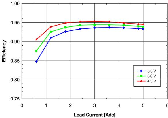
**Fig. 3.3V.3:** Efficiency vs. load current and input voltage for  $V_{out} = 3.3\text{ V}$  converter mounted vertically with air flowing from pin 5 to pin 1 at a rate of 200 LFM (1 m/s) and  $T_a = 25\text{ }^{\circ}\text{C}$ .
