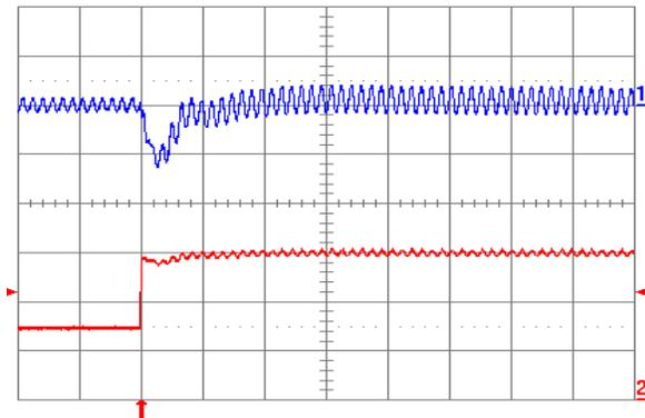
Fig. 1.8V.7: Output voltage response for  $V_{out} = 1.8\text{ V}$  to positive load current step change from 2.5 A to 5 A with slew rate of  $5\text{ A}/\mu\text{s}$  at  $V_{in} = 5\text{ V}$ . Top trace: output voltage (100 mV/div.); Bottom trace: load current (2 A/div.).  $C_o = 47\text{ }\mu\text{F}$  ceramic +  $1\text{ }\mu\text{F}$  ceramic. Time scale: 20  $\mu\text{s}$ /div.
