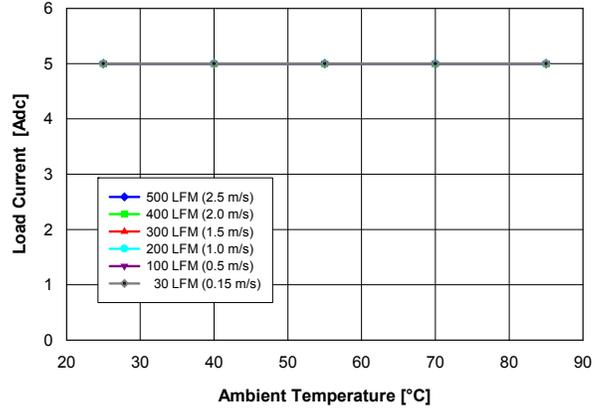
**Fig. 1.8V.2:** Available load current vs. ambient temperature and airflow rates for  $V_{out} = 1.8\text{ V}$  converter mounted horizontally with  $V_{in} = 5\text{ V}$ , air flowing from pin 5 to pin 1, and maximum MOSFET temperature  $\leq 120\text{ }^{\circ}\text{C}$ .
