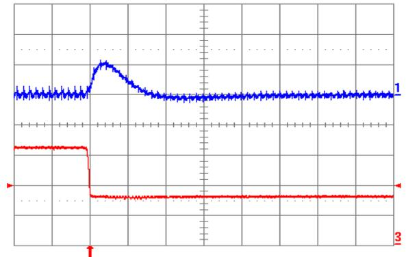
**Fig. 2.5V.7:** Output voltage response for  $V_{out} = 2.5\text{ V}$  to negative load current step change from 16 A to 8 A with slew rate of  $-5\text{ A}/\mu\text{s}$  at  $V_{in} = 12\text{ V}$ . Top trace: output voltage (200 mV/div.); Bottom trace: load current (5 A/div.).  $C_o = 100\ \mu\text{F}$  ceramic. Time scale: 20  $\mu\text{s}$ /div.
