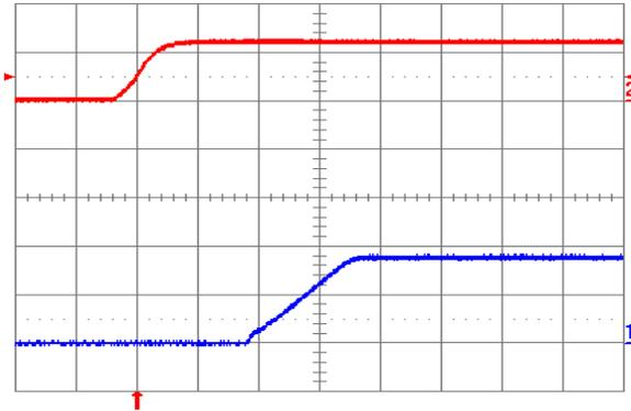
**Fig. 1.8V.4:** Turn-on transient for  $V_{out} = 1.8\text{ V}$  with application of  $V_{in}$  at full rated load current (resistive) and  $100\ \mu\text{F}$  external capacitance at  $V_{in} = 12\text{ V}$ . Top trace:  $V_{in}$  (10 V/div.); Bottom trace: output voltage (1 V/div.); Time scale: 2 ms/div.
