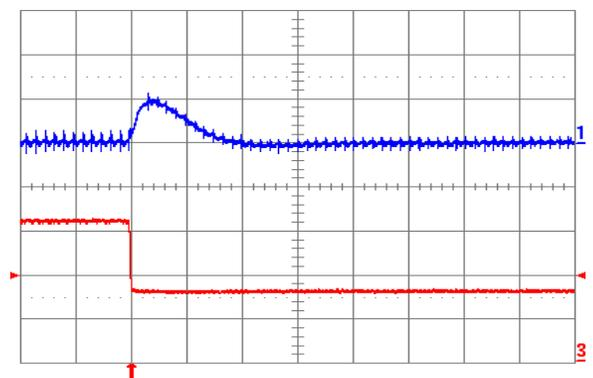
**Fig. 1.8V.7:** Output voltage response for  $V_{out} = 1.8\text{ V}$  to negative load current step change from 16 A to 8 A with slew rate of  $-5\text{ A}/\mu\text{s}$  at  $V_{in} = 12\text{ V}$ . Top trace: output voltage (200 mV/div.); Bottom trace: load current (5 A/div.).  $C_o = 100\ \mu\text{F}$  ceramic. Time scale: 20  $\mu\text{s}$ /div.
