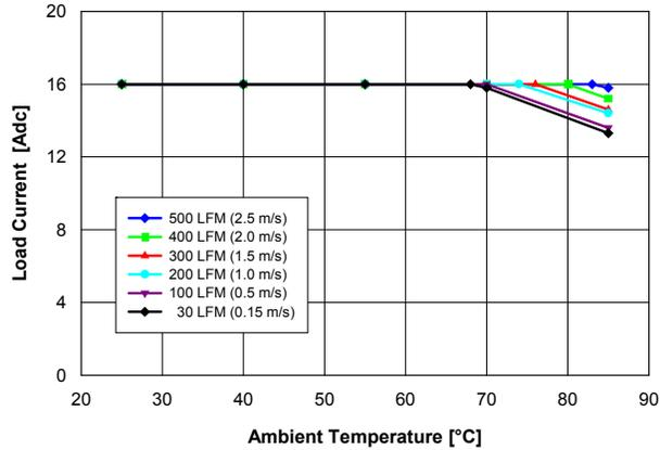
**Fig. 5.0V.1:** Available load current vs. ambient temperature and airflow rates for  $V_{out} = 5.0$  V converter mounted vertically with  $V_{in} = 12$  V, and maximum MOSFET temperature  $\leq 120$  °C.
