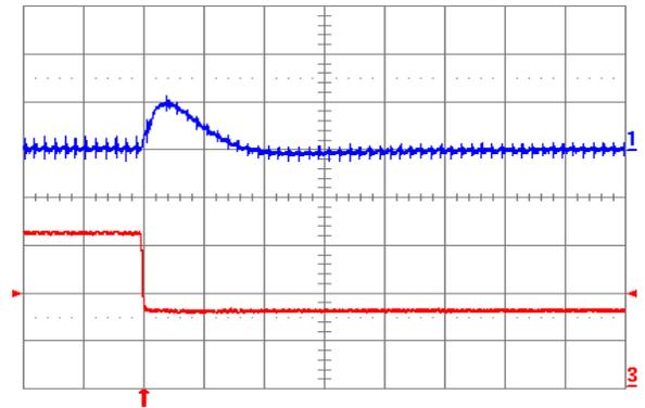
**Fig. 1.5V.7:** Output voltage response for  $V_{out} = 1.5\text{ V}$  to negative load current step change from 16 A to 8 A with slew rate of  $-5\text{ A}/\mu\text{s}$  at  $V_{in} = 12\text{ V}$ . Top trace: output voltage (200 mV/div.); Bottom trace: load current (5 A/div.).  $C_o = 100\ \mu\text{F}$  ceramic. Time scale: 20  $\mu\text{s}$ /div.
