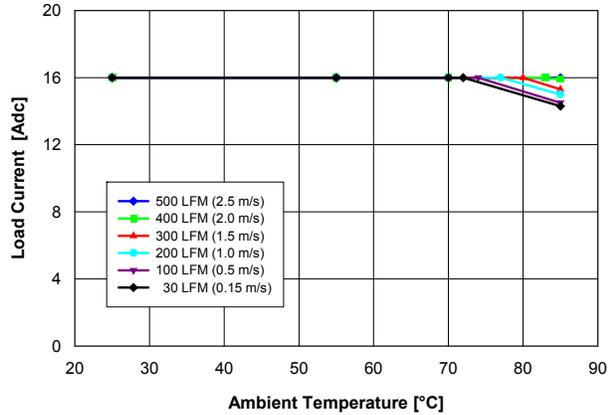
**Fig. 1.2V.1:** Available load current vs. ambient temperature and airflow rates for  $V_{out} = 1.2$  V converter mounted vertically with  $V_{in} = 12$  V, and maximum MOSFET temperature  $\leq 120$  °C.
