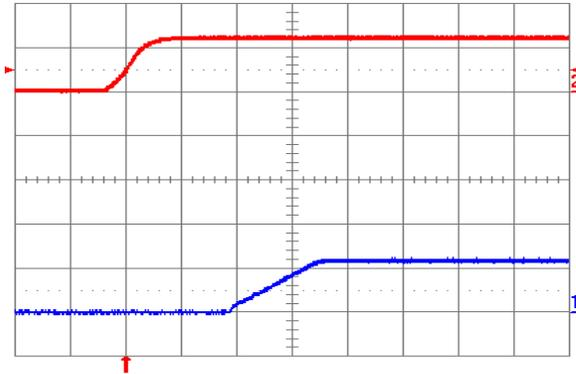
**Fig. 1.2V.4:** Turn-on transient for  $V_{out} = 1.2$  V with application of  $V_{in}$  at full rated load current (resistive) and  $100 \mu\text{F}$  external capacitance at  $V_{in} = 12$  V. Top trace:  $V_{in}$  (10 V/div.); Bottom trace: output voltage (1 V/div.); Time scale: 2 ms/div.
