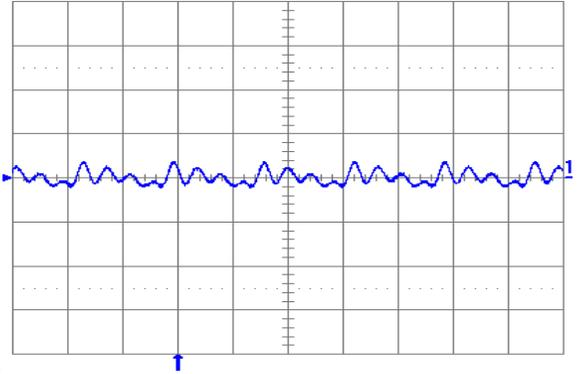
**Fig. 1.2V.5:** Output voltage ripple (20 mV/div.) at full rated load current into a resistive load with external capacitance  $100 \mu\text{F}$  ceramic +  $1 \mu\text{F}$  ceramic and  $V_{in} = 12$  V for  $V_{out} = 1.2$  V. Time scale: 2  $\mu\text{s}$ /div.
