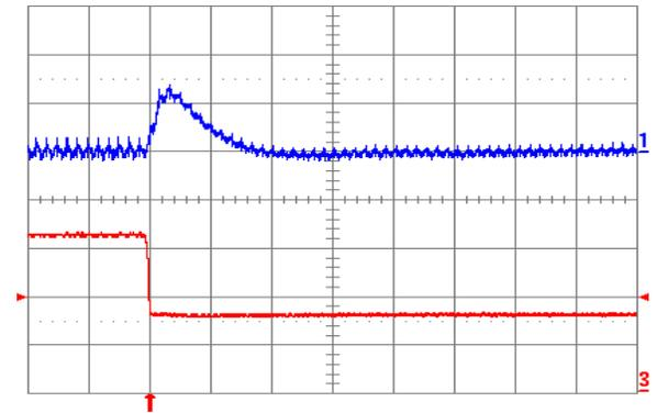
**Fig. 5.0V.7:** Output voltage response for  $V_{out} = 5.0$  V to negative load current step change from 16 A to 8 A with slew rate of  $-5 \text{A}/\mu\text{s}$  at  $V_{in} = 12$  V. Top trace: output voltage (200 mV/div.); Bottom trace: load current (5A/div.).  $C_o = 100 \mu\text{F}$  ceramic. Time scale: 20  $\mu\text{s}$ /div.
