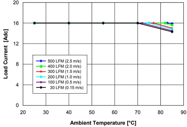
**Fig. 1.8V.1:** Available load current vs. ambient temperature and airflow rates for  $V_{out} = 1.8$  V converter mounted vertically with  $V_{in} = 12$  V, and maximum MOSFET temperature  $\leq 120$  °C.
