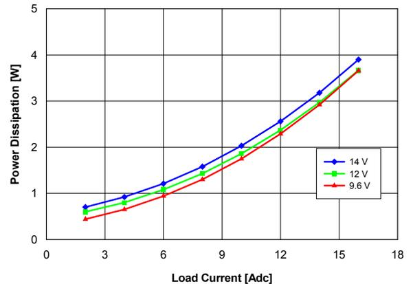
**Fig. 1.2V.3:** Power loss vs. load current and input voltage for  $V_{out} = 1.2$  V converter mounted vertically with air flowing at a rate of 200 LFM (1 m/s) and  $T_a = 25$  °C.
