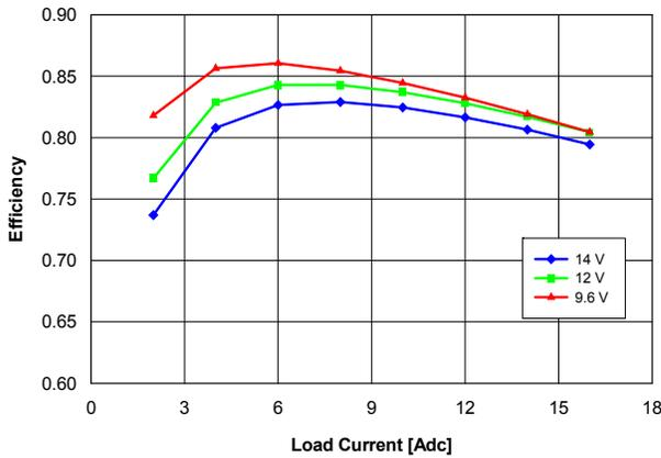
**Fig. 1.0V.2:** Efficiency vs. load current and input voltage for V<sub>out</sub> = 1.0 V converter mounted vertically with air flowing at a rate of 200 LFM (1 m/s) and T<sub>a</sub> = 25 °C.
