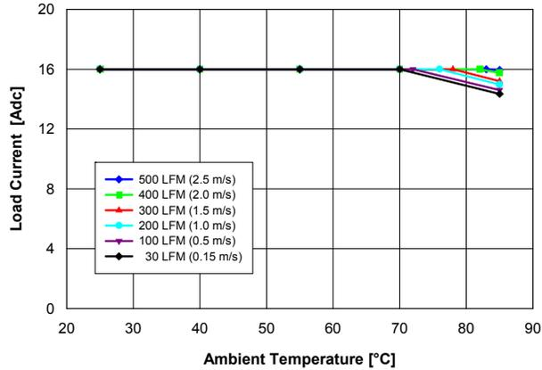
**Fig. 2.0V.1:** Available load current vs. ambient temperature and airflow rates for  $V_{out} = 2.0$  V converter mounted vertically with  $V_{in} = 12$  V, and maximum MOSFET temperature  $\leq 120$  °C.
