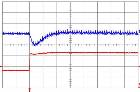
**Fig. 2.5V.6:** Output voltage response for  $V_{out} = 2.5\text{ V}$  to positive load current step change from 8 A to 16 A with slew rate of  $5\text{ A}/\mu\text{s}$  at  $V_{in} = 12\text{ V}$ . Top trace: output voltage (200 mV/div.); Bottom trace: load current (5 A/div.).  $C_o = 100\ \mu\text{F}$  ceramic. Time scale: 20  $\mu\text{s}$ /div.
