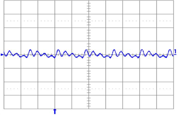
**Fig. 1.0V.5:** Output voltage ripple (20 mV/div.) at full rated load current into a resistive load with external capacitance  $100 \mu\text{F}$  ceramic +  $1 \mu\text{F}$  ceramic and  $V_{in} = 12$  V for  $V_{out} = 1.0$  V. Time scale: 2  $\mu\text{s}$ /div.
