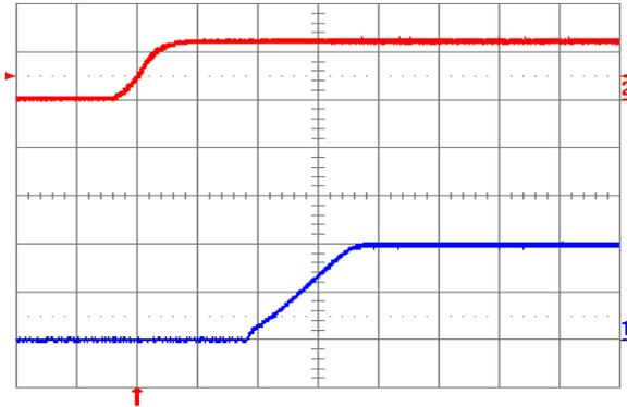
**Fig. 2.0V.4:** Turn-on transient for  $V_{out} = 2.0$  V with application of  $V_{in}$  at full rated load current (resistive) and  $100 \mu\text{F}$  external capacitance at  $V_{in} = 12$  V. Top trace:  $V_{in}$  (10 V/div.); Bottom trace: output voltage (1 V/div.); Time scale: 2 ms/div.
