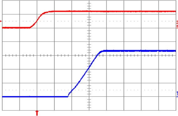
**Fig. 3.3V.4:** Turn-on transient for  $V_{out} = 3.3\text{ V}$  with application of  $V_{in}$  at full rated load current (resistive) and  $100\ \mu\text{F}$  external capacitance at  $V_{in} = 12\text{ V}$ . Top trace:  $V_{in}$  (10 V/div.); Bottom trace: output voltage (1 V/div.); Time scale: 2 ms/div.
