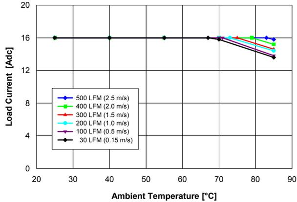
**Fig. 3.3V.1:** Available load current vs. ambient temperature and airflow rates for  $V_{out} = 3.3$  V converter mounted vertically with  $V_{in} = 12$  V, and maximum MOSFET temperature  $\leq 120$  °C.
