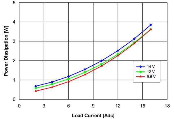
**Fig. 1.0V.3:** Power loss vs. load current and input voltage for V<sub>out</sub> = 1.0 V converter mounted vertically with air flowing at a rate of 200 LFM (1 m/s) and T<sub>a</sub> = 25 °C.
