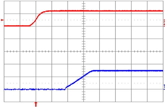
**Fig. 1.5V.4:** Turn-on transient for  $V_{out} = 1.5\text{ V}$  with application of  $V_{in}$  at full rated load current (resistive) and  $100\ \mu\text{F}$  external capacitance at  $V_{in} = 12\text{ V}$ . Top trace:  $V_{in}$  (10 V/div.); Bottom trace: output voltage (1 V/div.); Time scale: 2 ms/div.
