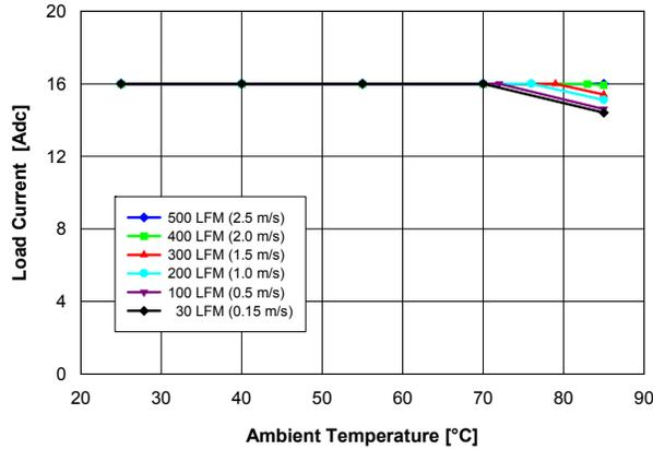
**Fig. 0.7525V.1:** Available load current vs. ambient temperature and airflow rates for  $V_{out} = 1.0$  V converter mounted vertically with  $V_{in} = 12$  V, and maximum MOSFET temperature  $\leq 120$  °C.
