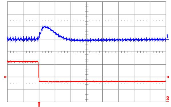
**Fig. 2.0V.7:** Output voltage response for  $V_{out} = 2.0$  V to negative load current step change from 16 A to 8 A with slew rate of  $-5 \text{ A}/\mu\text{s}$  at  $V_{in} = 12$  V. Top trace: output voltage (200 mV/div.); Bottom trace: load current (5 A/div.).  $C_o = 100 \mu\text{F}$  ceramic. Time scale: 20  $\mu\text{s}$ /div.
