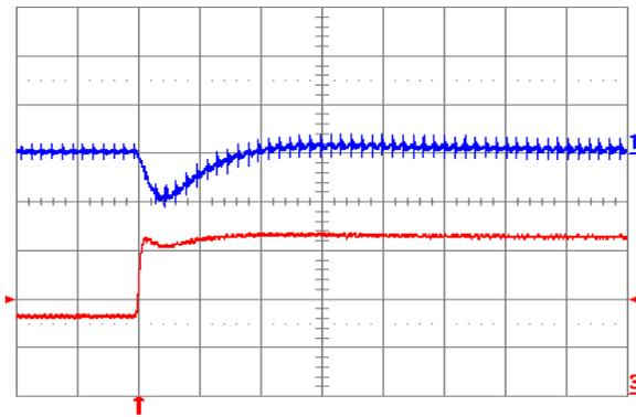
**Fig. 1.2V.6:** Output voltage response for  $V_{out} = 1.2$  V to positive load current step change from 8 A to 16 A with slew rate of  $5 \text{ A}/\mu\text{s}$  at  $V_{in} = 12$  V. Top trace: output voltage (200 mV/div.); Bottom trace: load current (5 A/div.).  $C_o = 100 \mu\text{F}$  ceramic. Time scale: 20  $\mu\text{s}$ /div.
