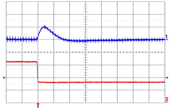
**Fig. 1.2V.7:** Output voltage response for  $V_{out} = 1.2$  V to negative load current step change from 16 A to 8 A with slew rate of  $-5 \text{ A}/\mu\text{s}$  at  $V_{in} = 12$  V. Top trace: output voltage (200 mV/div.); Bottom trace: load current (5 A/div.).  $C_o = 100 \mu\text{F}$  ceramic. Time scale: 20  $\mu\text{s}$ /div.
