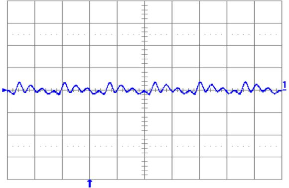
**Fig. 0.7525V.5:** Output voltage ripple (20 mV/div.) at full rated load current into a resistive load with external capacitance  $100\ \mu\text{F}$  ceramic +  $1\ \mu\text{F}$  ceramic and  $V_{in} = 12\ \text{V}$  for  $V_{out} = 0.7525\ \text{V}$ . Time scale: 2  $\mu\text{s}$ /div.
