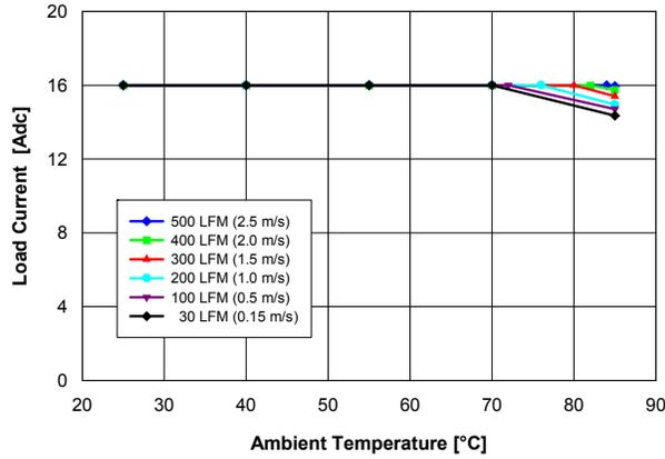
**Fig. 1.0V.1:** Available load current vs. ambient temperature and airflow rates for V<sub>out</sub> = 1.0 V converter mounted vertically with V<sub>in</sub> = 12 V, and maximum MOSFET temperature ≤ 120 °C.
