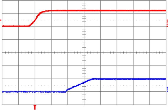
**Fig. 1.0V.4:** Turn-on transient for  $V_{out} = 1.0$  V with application of  $V_{in}$  at full rated load current (resistive) and  $100 \mu\text{F}$  external capacitance at  $V_{in} = 12$  V. Top trace:  $V_{in}$  (10 V/div.); Bottom trace: output voltage (1 V/div.); Time scale: 2 ms/div.
